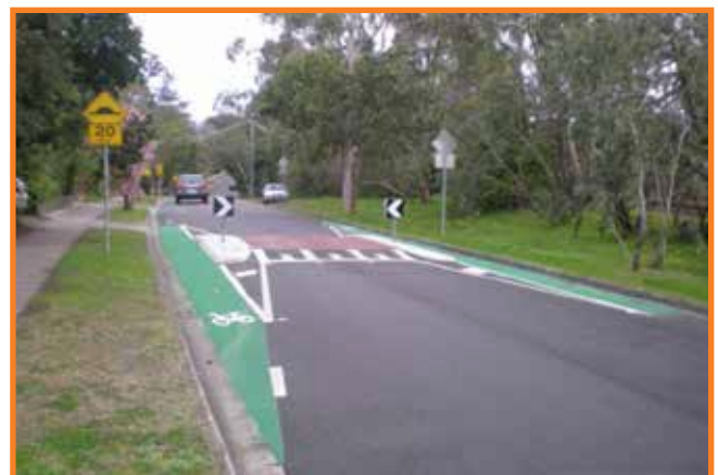
One-way slow point with bicycle-bypass facilities 3
