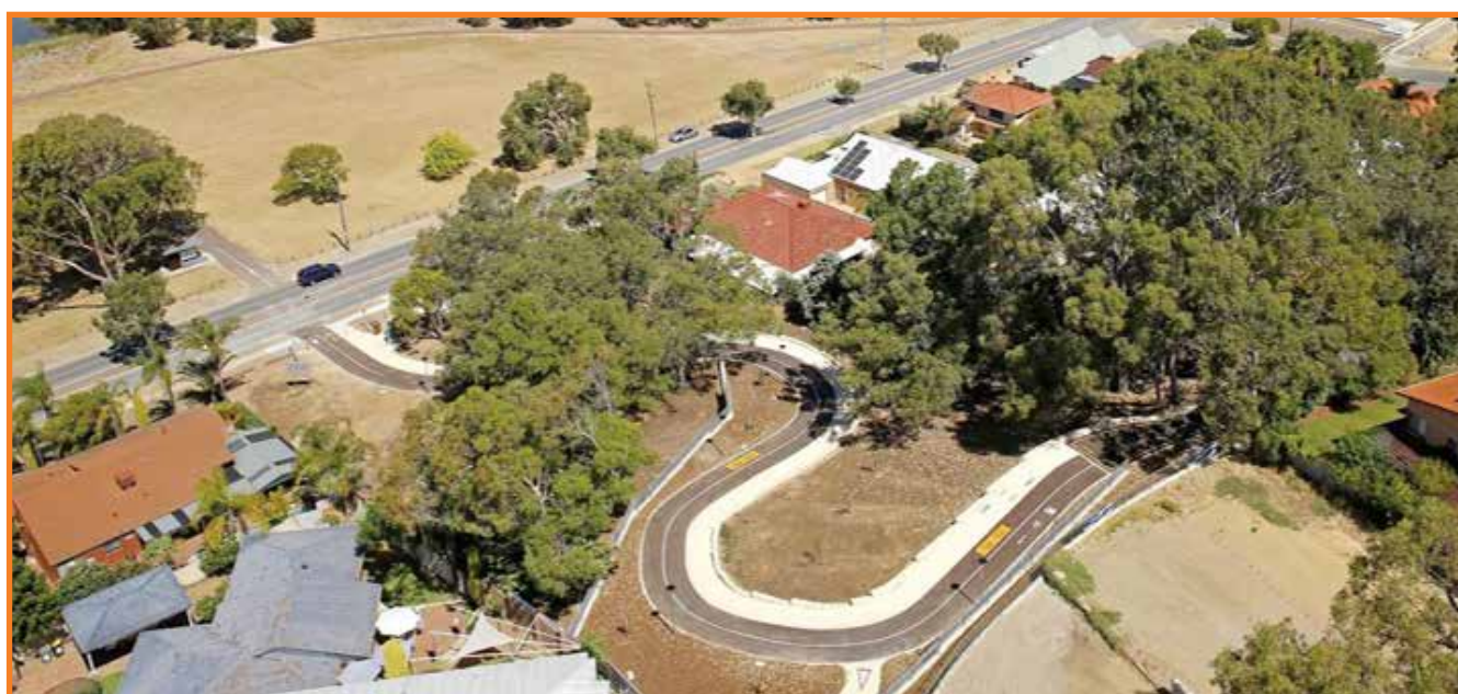
Figure 4.16 Zig-zags positioned in appropriate locations could be used to help cyclists overcome Geraldton's steep gradients.
