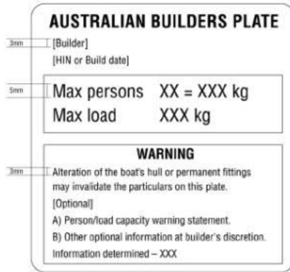
Figure 6 — Sample ABP template for boats 6 metres or more in length, not designed to be powered by an outboard engine
