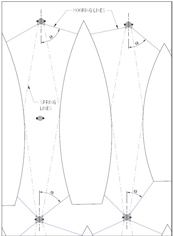
Figure 1: Minimum recommended Mooring Guideline for vessels using "Sticks" Pens in Cyclonic Conditions Note: Vessels must be moored directly on the piles using the mooring rings provided.
