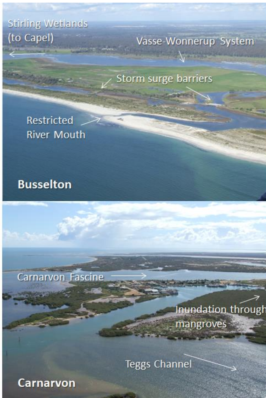
Figure 4-3: Inundation Pathways for Busselton/Capel and Carnarvon Inundation hazard for each townsite may arrive through multiple pathways. For Busselton and Capel, a key pathway for inundation hazard is through narrow river and agricultural channels. At Carnarvon, inundation may arrive through waterways, or overland, through the mangrove flats.
