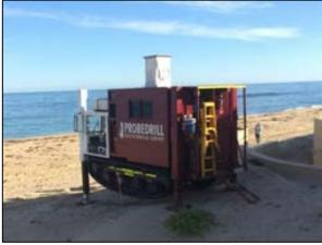
Figure 5: CPT data acquisition during a previous coastal investigation.
