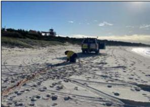
Figure 3: MASW data acquisition using a seismic streamer.
