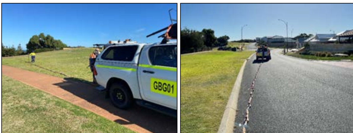
Figure 3: MASW data acquisition using a seismic streamer.
