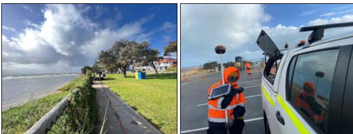
Figure 3: MASW data acquisition using a seismic streamer.
