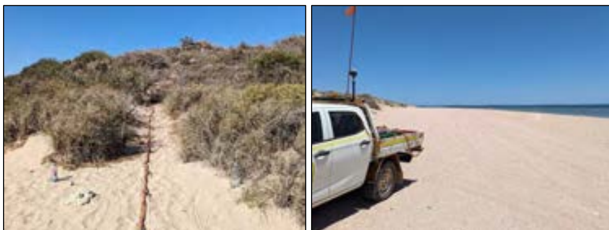
Figure 4: MASW data acquisition using a seismic streamer.
