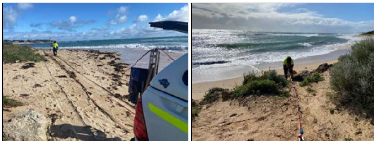
Figure 3: MASW data acquisition using a seismic streamer.
