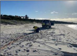
Figure 3: MASW data acquisition using a seismic streamer.
