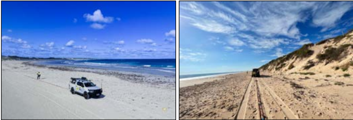
Figure 3: MASW data acquisition using a seismic streamer.
