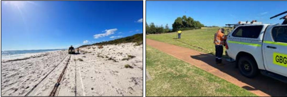
**Figure 3: MASW data acquisition using a seismic streamer.**
