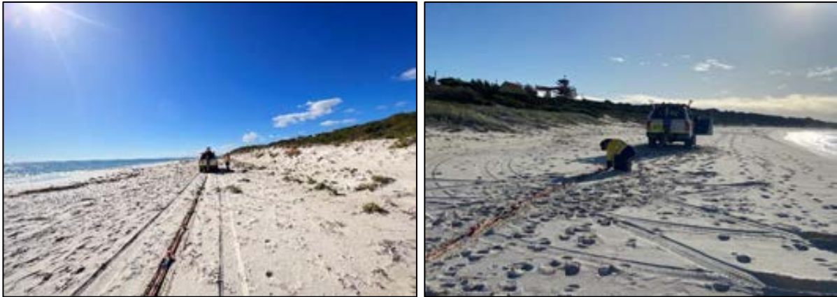
Figure 3: MASW data acquisition using a seismic streamer.
