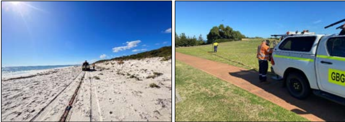
Figure 3: MASW data acquisition using a seismic streamer.
