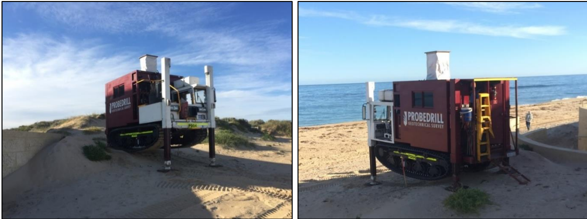
Figure 5: CPT data acquisition during a previous coastal investigation.
