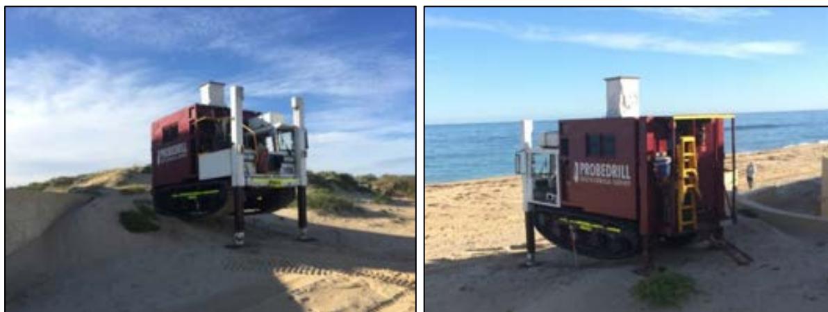
Figure 5: CPT data acquisition during a previous coastal investigation.
