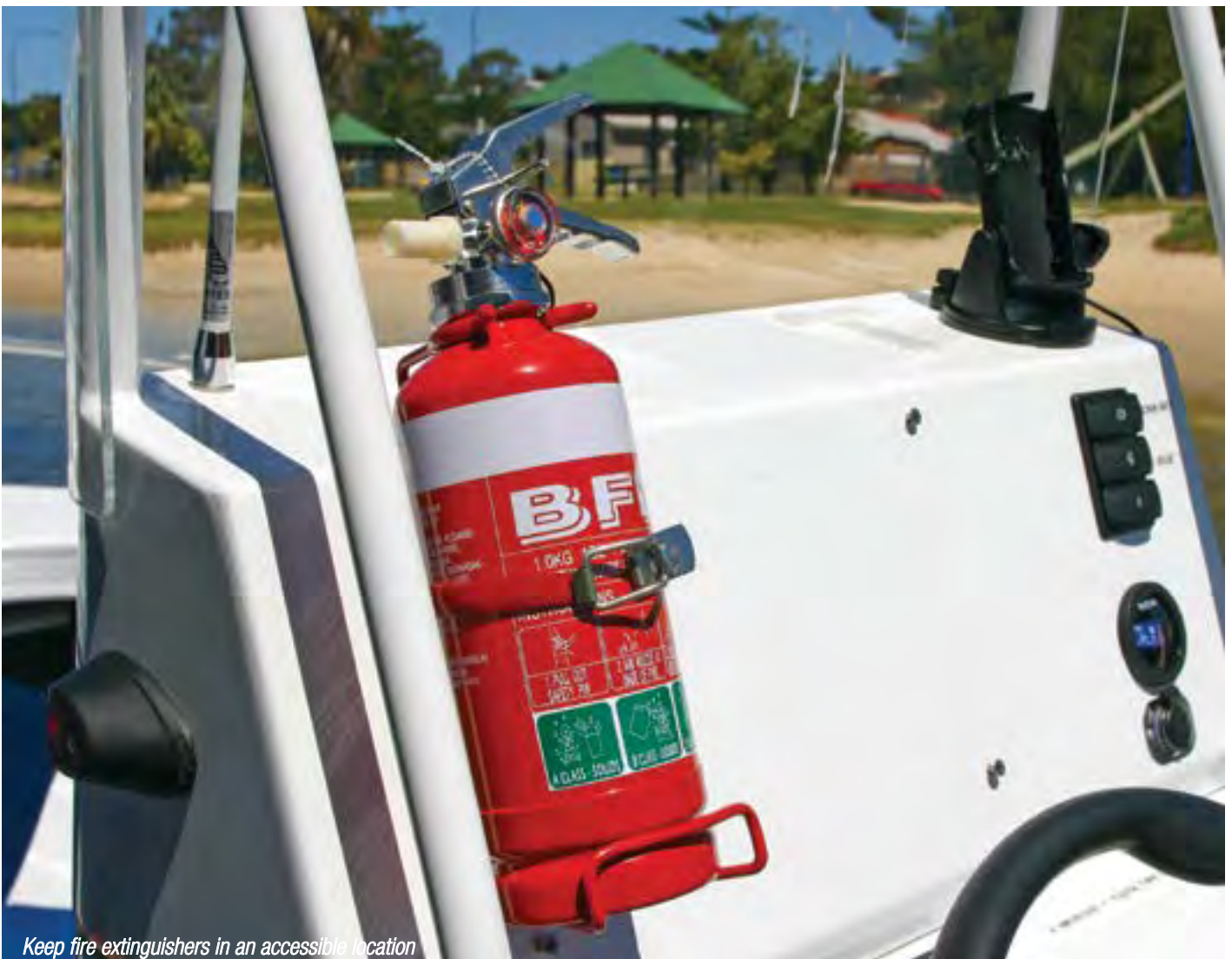
Check the gauge is in the green
