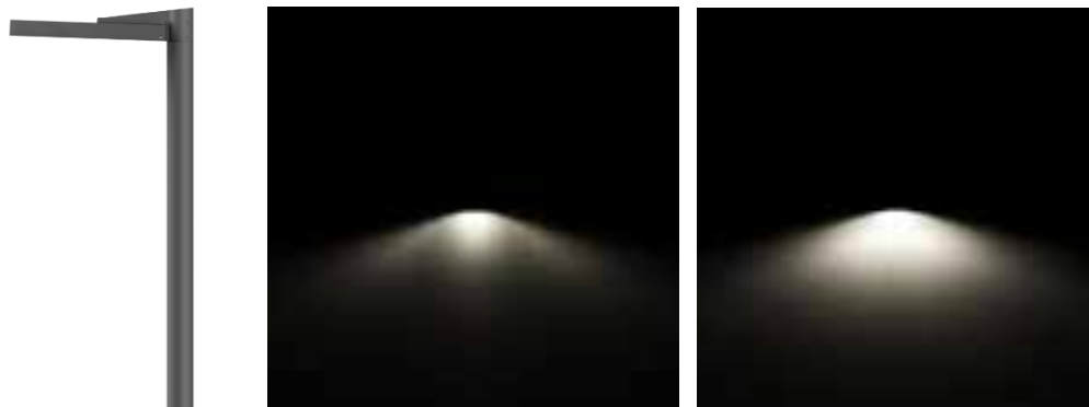
Figure 4: WE-EF VFL530-SE 26W light and IES light distribution. Source: https://www.we-ef.com/aus
