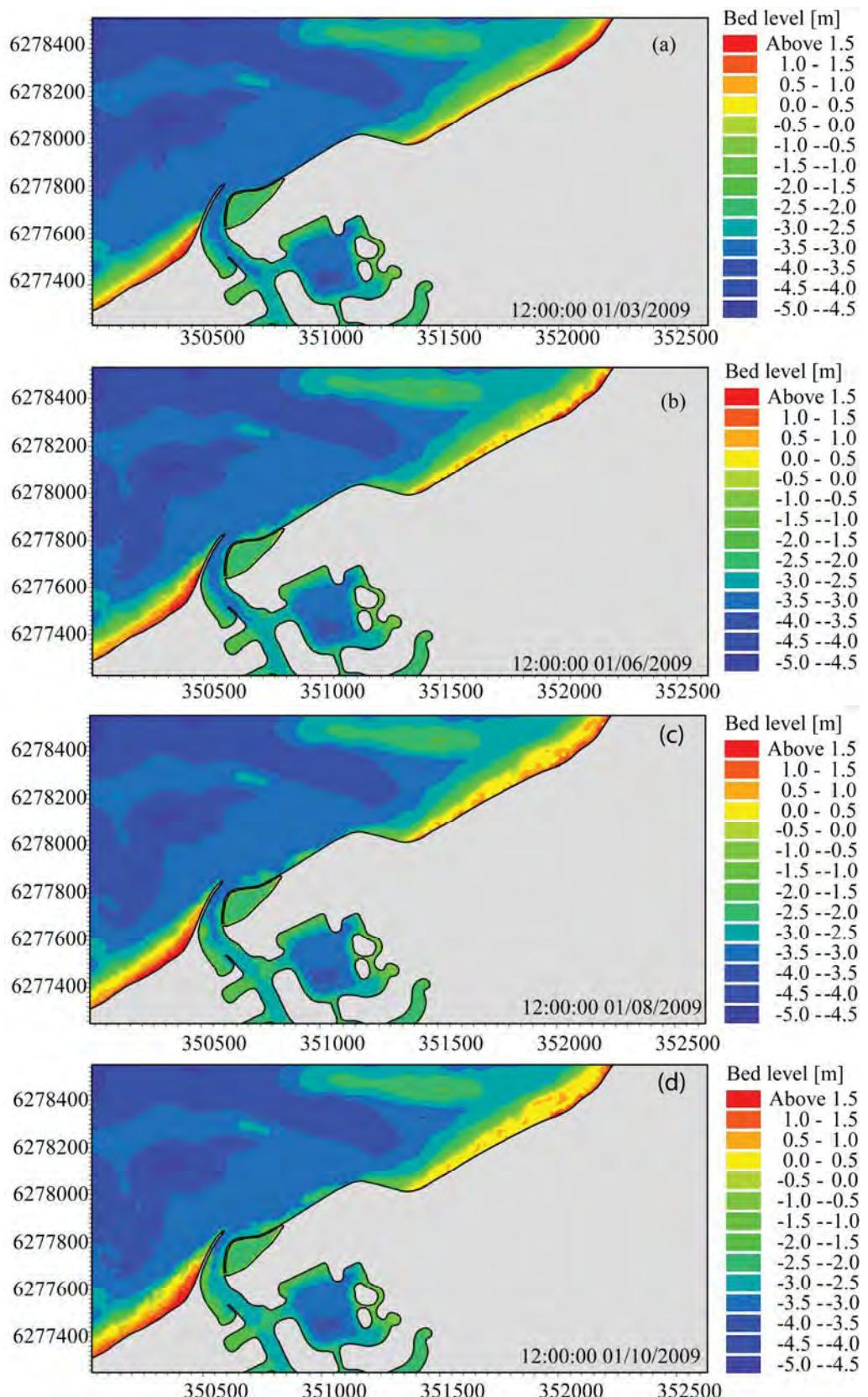
**Figure 4.79 Model-predicted bed levels in the vicinity of Port Geographe for Scenario 7. (a) Model initial bathymetry on 01 March 2009 and predicted bed levels on (b) 1 June 2009; (c) 1 August 2009; and, (d) 1 October 2009.**
