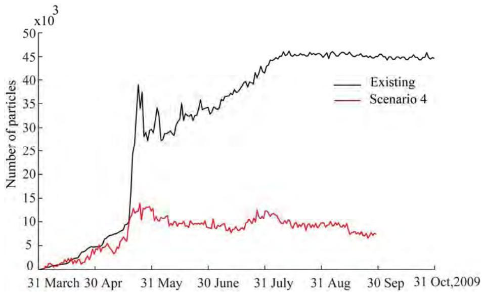
**Figure 4.60 Predicted cumulative number of particles (seagrass wrack) at the western beach, Port Geographe from March to October 2009 for Scenario 4.**
