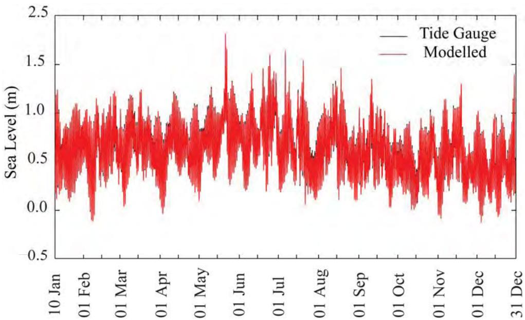
**Figure 3.1 Measured and predicted water levels at the Busselton tide station in 2009. Black lines denote observed data and red lines denote model output.**
