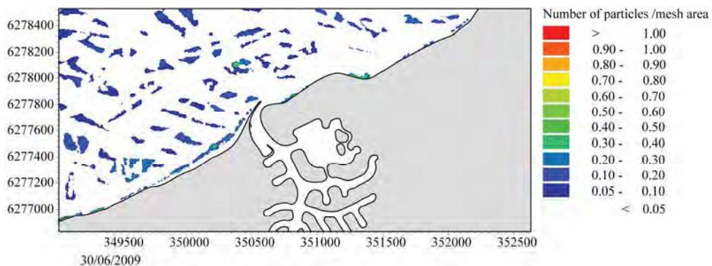
**Figure 4.66 Particle distribution in the vicinity of Port Geographe on 30 June 2009 for Scenario 5.**
