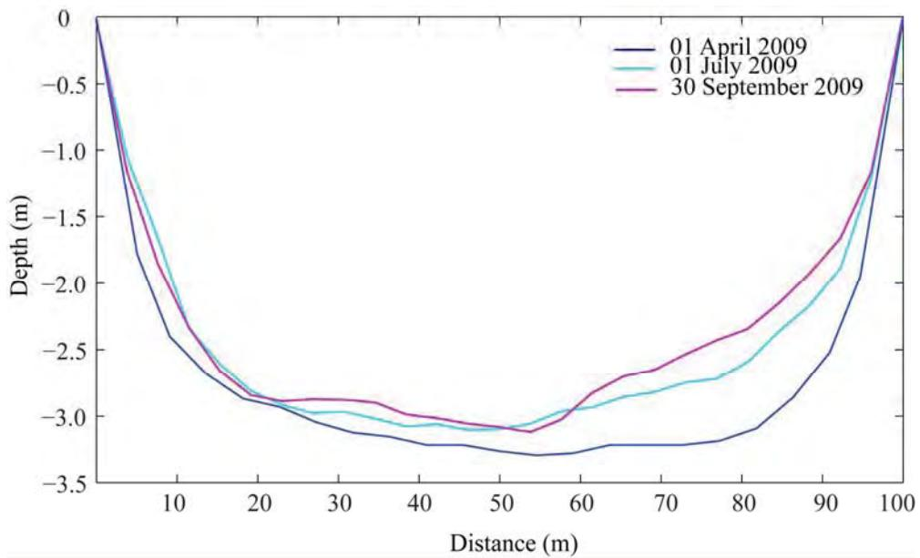
**Figure 4.56 Predicted bed levels across the harbour entrance channel (Cross-section x-y) of Port Geographe for Scenario 4 from 01 March to 30 October 2009.**
