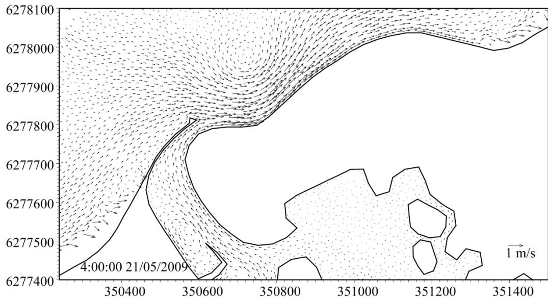
**Figure 4.30** Model-predicted current pattern in the vicinity of Port Geographe for Scenario 2 (Option 5a) during a storm event (0400 hr, 21 May 2009).
