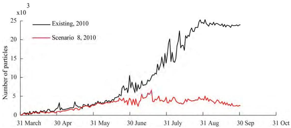
**Figure 4.100 A comparison of Scenario 8 and existing condition predicted cumulative number of particle (seagrass wrack) at the western beach, Port Geographe for 2010.**
