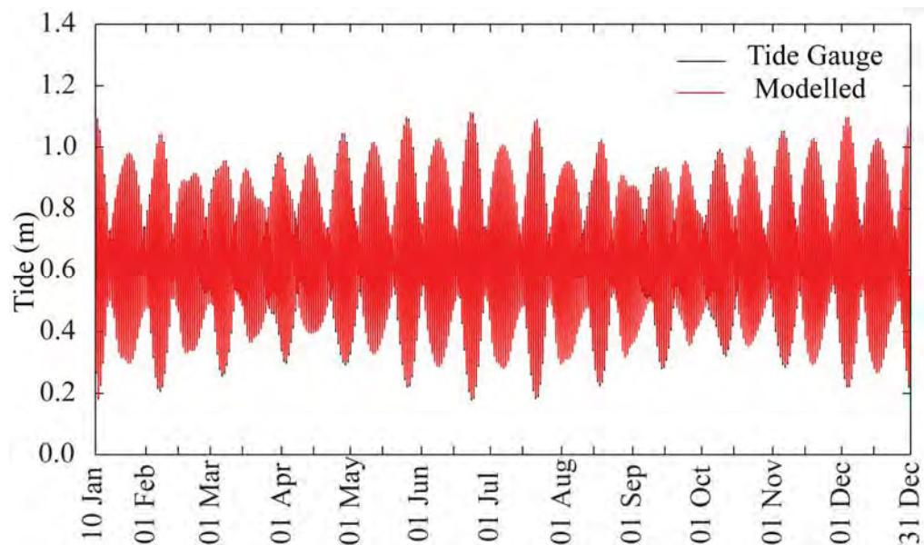
**Figure 3.2 Measured and predicted tides at the Busselton tide station in 2009. Black lines denote observed data and red lines denote model output.**
