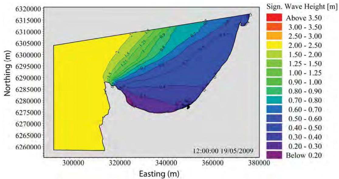
**Figure 4.12 Snapshot of predicted wave height distribution before a storm event (on 19 May 2009).**
