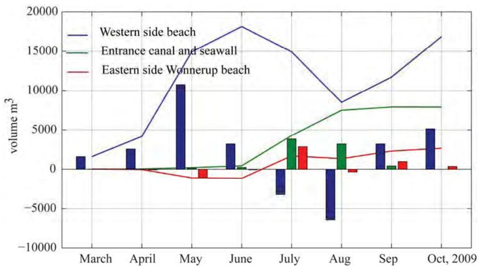
**Figure 4.89 Model-simulated monthly sand accretion and cumulative volume during 01 March to 30 October 2009 at different locations of Port Geographe for Scenario 8.**
