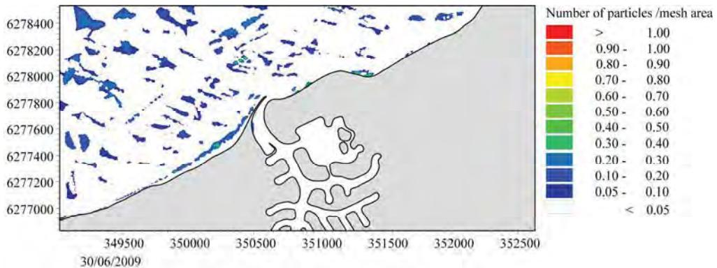
**Figure 4.58. Particle distribution in the vicinity of Port Geographe on 30 June 2009 for Scenario 4.**
