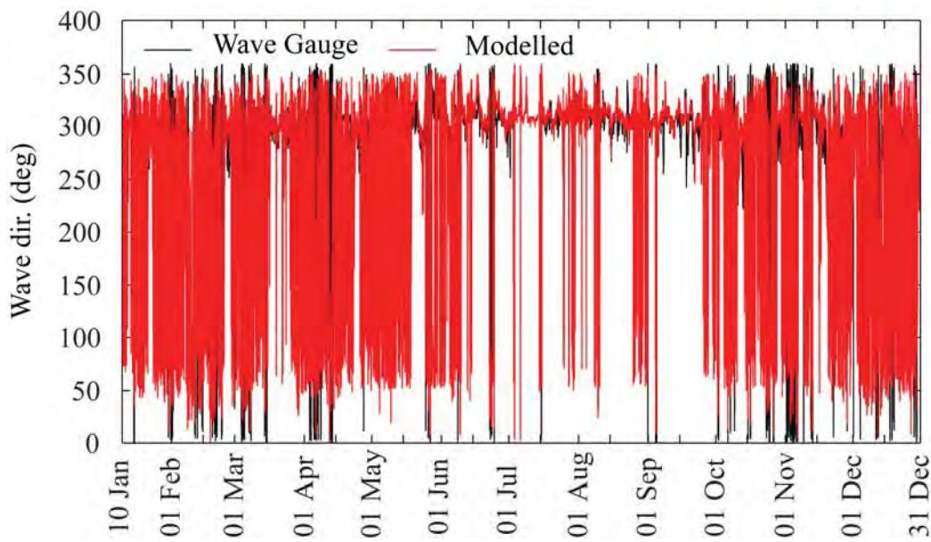
**Figure 3.8 Measured and predicted mean wave direction at the AWAC site in 2009.**
