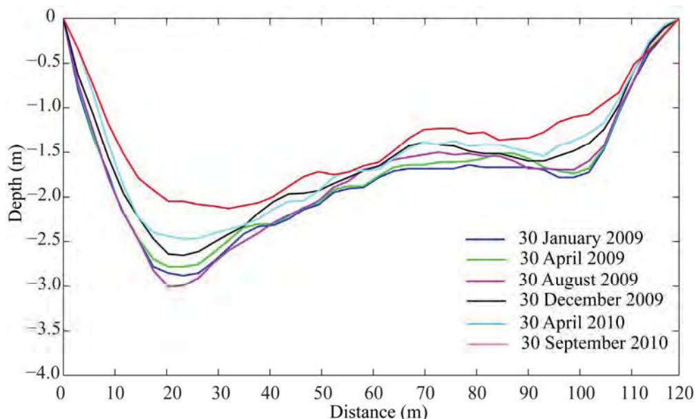
**Figure 4.22 Predicted bed levels across the entrance channel (section A-B) of Port Geographe from January 2009 to September 2010.**
