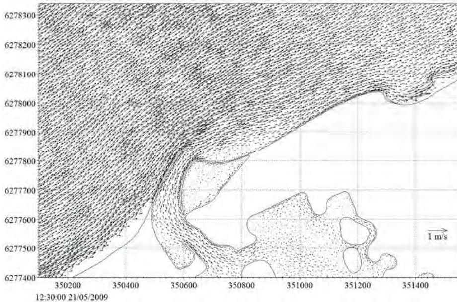
**Figure 4.102** Snapshot of predicted current pattern in the Port Geographe area at the peak of storm on May 21 2009 for the Scenario 8.
