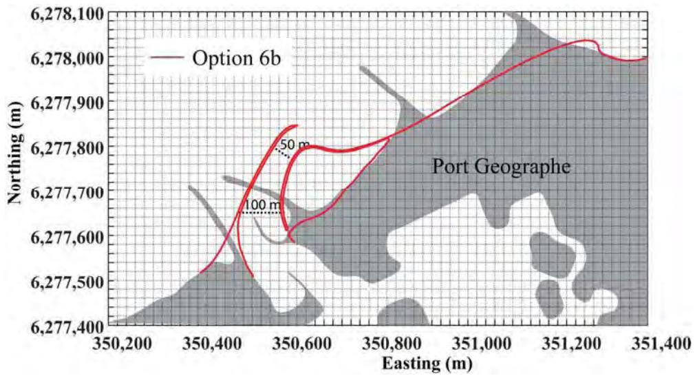
**Figure 4.85 Scenario 8 layout of Port Geographe. Black dotted line shows existing Port Geographe layout and red solid lines shows layout of Scenario 8.**
