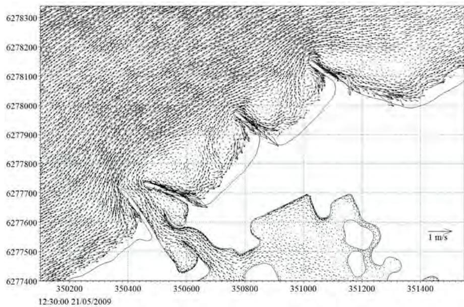
**Figure 4.101** Snapshot of predicted current pattern in the Port Geographe area at the peak of storm on May 21 2009 for the existing groyne configuration.
