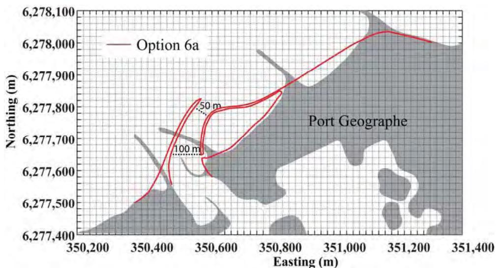
**Figure 4.77 Scenario 7 layout of Port Geographe. Black dotted line shows existing Port Geographe layout and red solid lines shows layout of Scenario 7.**
