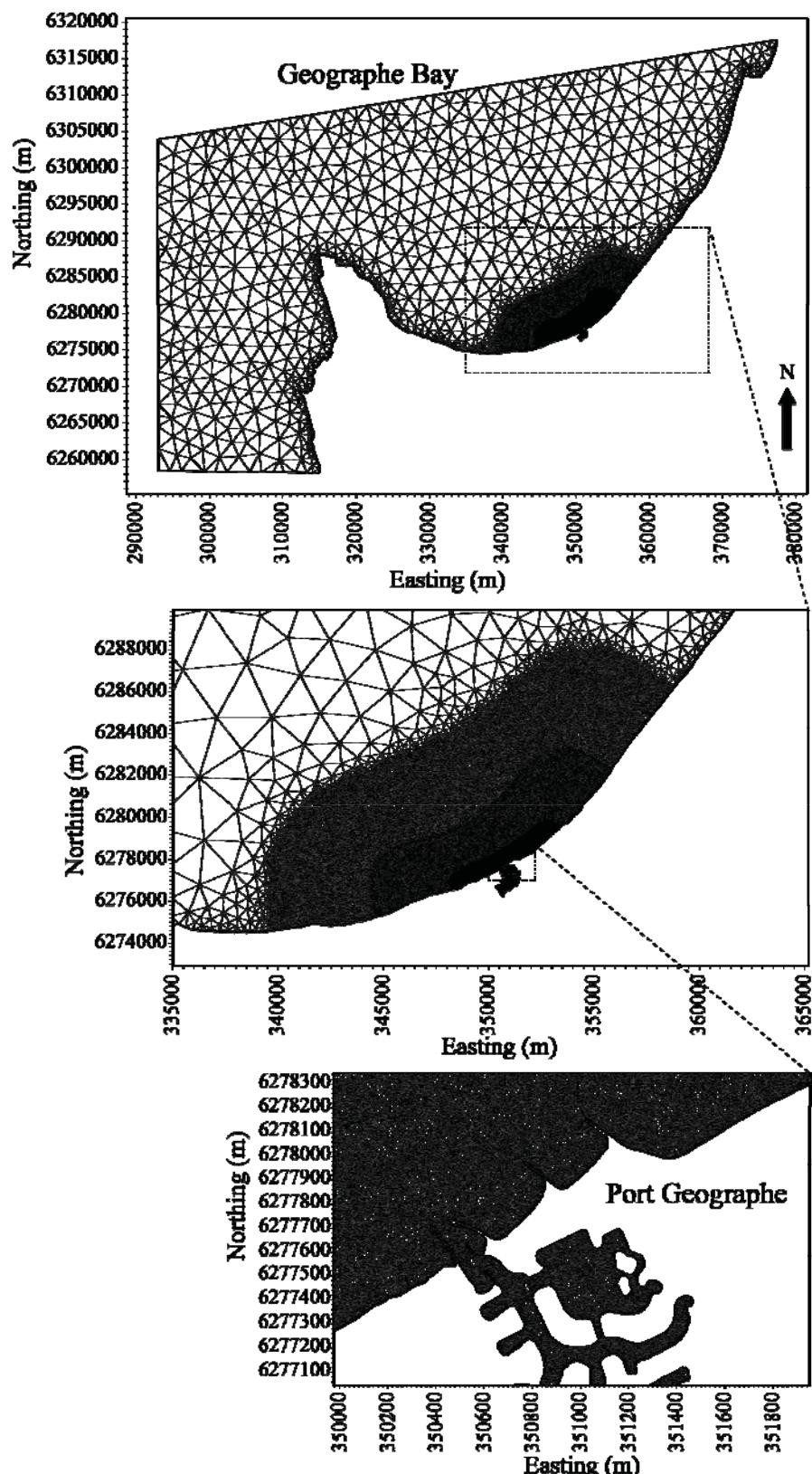
**Figure 2.5 Model mesh grid of Geographe Bay showing different scales used for the model domain. Fine grids are used in the Port Geographe and near shore regions of Geographe Bay.**
