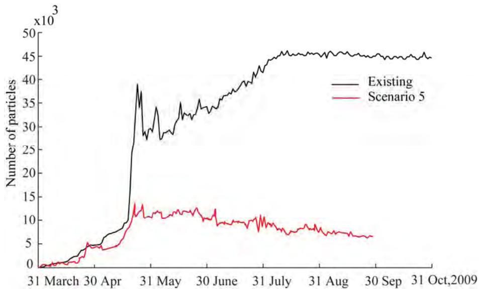
**Figure 4.68m Predicted cumulative number of particles (seagrass wrack) at the western beach, Port Geographe from March to October 2009 for Scenario 5.**
