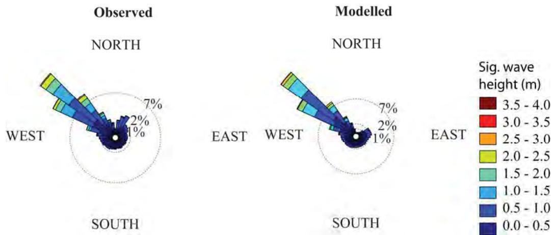
**Figure 3.10 Wave rose diagrams (in metres) based on measured and predicted wave climate parameters at AWAC site during 2009.**
