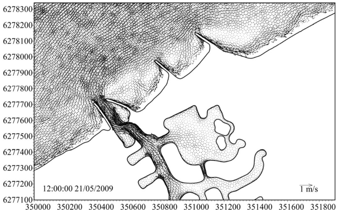
**Figure 4.11 Model-predicted velocity vector plots in the vicinity of Port Geographe at the peak of storm event (0400 hr, 21 May 2009).**
