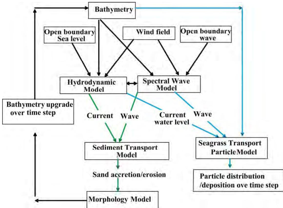
**Figure 2.1 Schematic of coupled numerical model flow diagram.**
