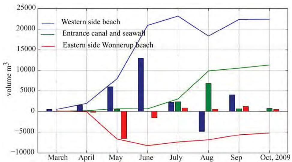
**Figure 4.73** Model-simulated monthly sand accretion and cumulative volume during 01 March to 30 October 2009 at different locations of Port Geographe for Scenario 6.
