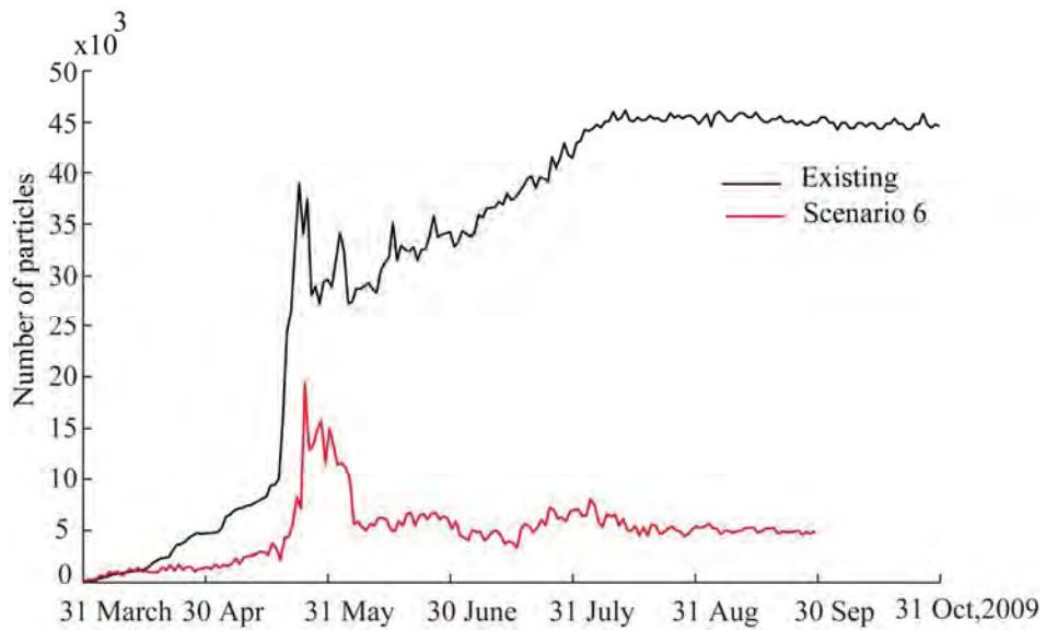
**Figure 4.76 Predicted cumulative number of particles (seagrass wrack) at the western beach, Port Geographe from March to October 2009 for Scenario 6.**
