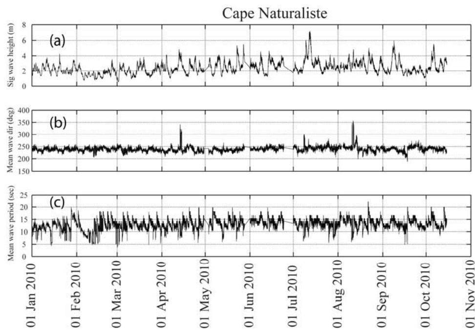
**Figure 4.7 Open boundary wave climate forcing data in 2010, obtained from the Cape Naturaliste Wave Buoy (source: Western Australian Department of Transport). (a) Significant wave height, (b) mean wave direction and (c) mean wave period.**
