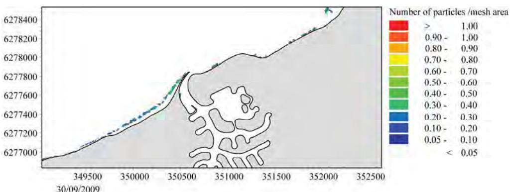
**Figure 4.59 Particle distribution in the vicinity of Port Geographe on 30 June 2009 for Scenario 4.**
