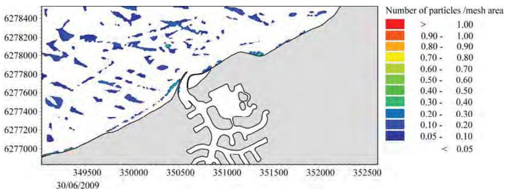
**Figure 4.82 Particle distribution in the vicinity of Port Geographe on 30 June 2009 for Scenario 7**
