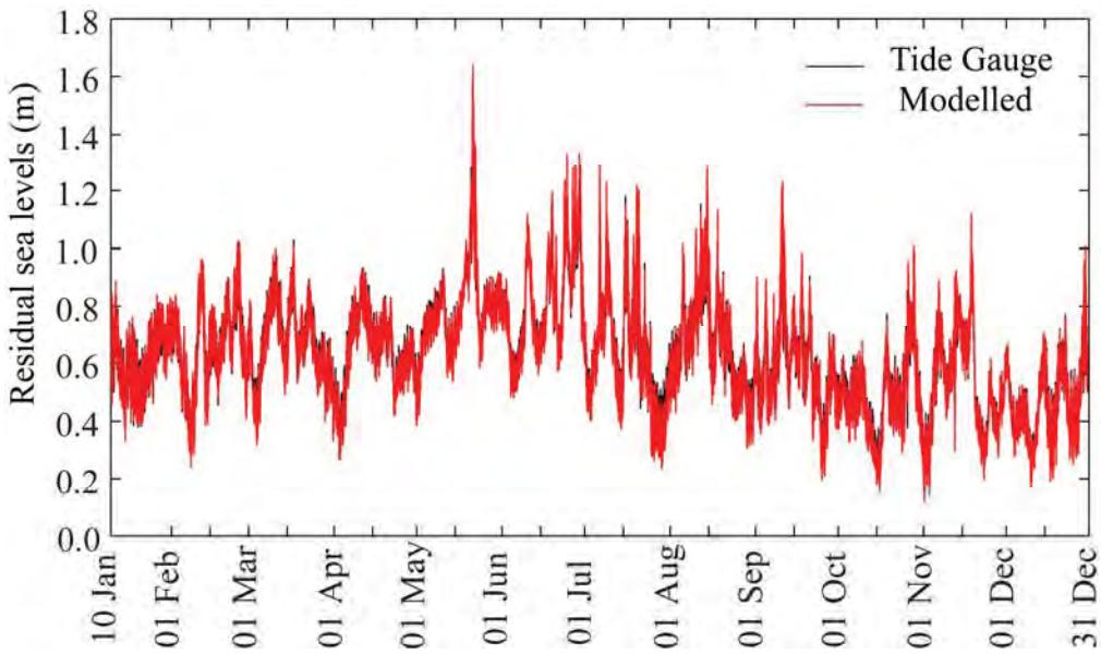
**Figure 3.3 Measured and predicted residual sea levels at the Busselton tide station in 2009. Black lines denote observed data and red lines denote model output.**
