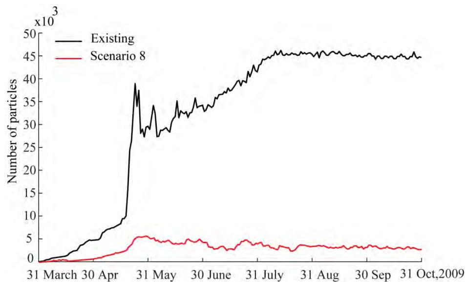
**Figure 4.95 A comparison of predicted cumulative number of particles (seagrass wrack) at the western beach, Port Geographe for Scenario 8 (under a repeat forcing of 2009).**
