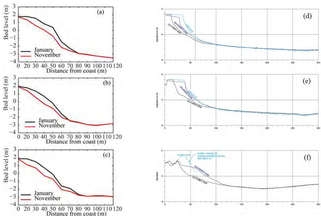
**Figure 3.26 Comparison between predicted and measured beach profiles in 2009 along Wonnerup Beach. (a) to (c) predicted profiles; (d) to (f) measured profiles (see Figure 3.24). (a) and (d) for section Ex1; (b) and (e) for section Ex2; and, (c) and (f) for section Ex3.**
