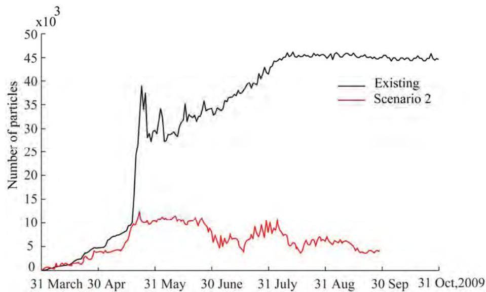
**Figure 4.42 Comparison of seagrass wrack accumulation and bypass between Scenario 2 and the existing configuration. The graph depicts the numbers of simulated cumulative particles from the model at the western beach, Port Geographe in 2009.**
