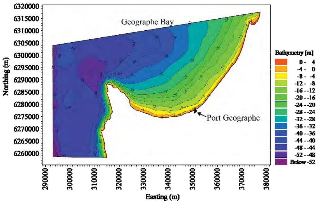
**Figure 2.3:** Initial model bathymetry of Geographe Bay in the current configuration.
