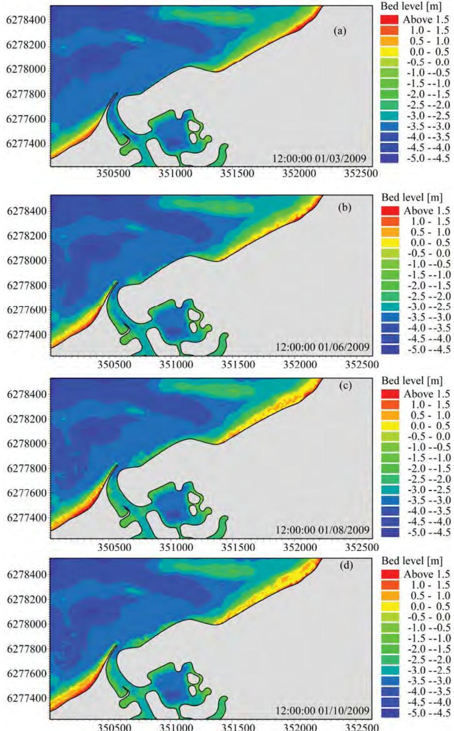
**Figure 4.63 Predicted bed levels in the vicinity of Port Geographe for Scenario 5. (a) Model initial bathymetry on 01 March 2009 and Predicted bed levels on: (b) 1 June 2009, (c) 1 August 2009 and (d) 1 October 2009.**
