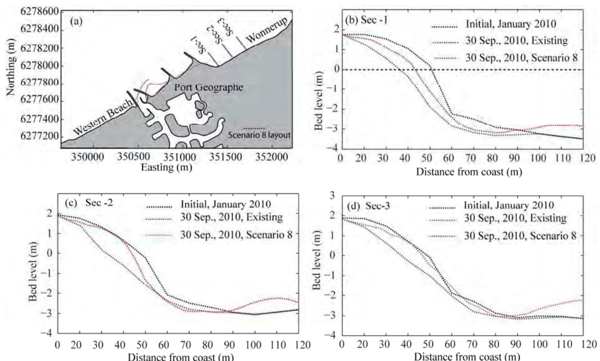
**Figure 4.105 Comparison of predicted bed level profiles along the Wonnerup beach for the existing configuration and Scenario 8. (a) location of cross-sections and predicted profiles for: (b) section 1 (Sec-1); (c) section 2 (Sec-2); and, (d) f section 3 (Sec-3)**
