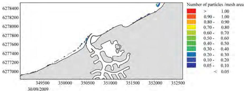
**Figure 4.91 Particle distribution in the vicinity of Port Geographe on 30 September 2009 for Scenario 8.**
