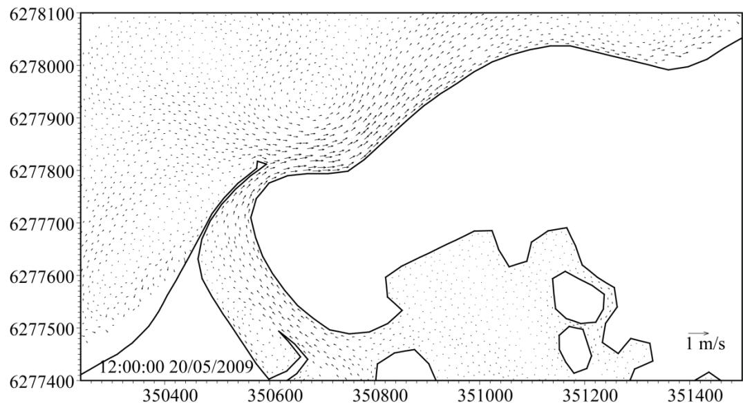
**Figure 4.29** Model-predicted current pattern in the vicinity of Port Geographe for Scenario 2 (Option 5a) at the beginning of a storm event (1200 hr, 20 May 2009).
