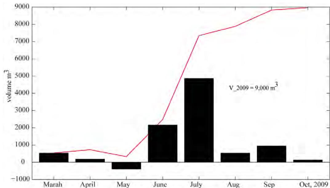
**Figure 4.40** Predicted monthly sand accretion and cumulative sand volume from 01 March to 01 November 2009 in front of seawall (see Figure 4.37 for selected area) under Scenario 2.
