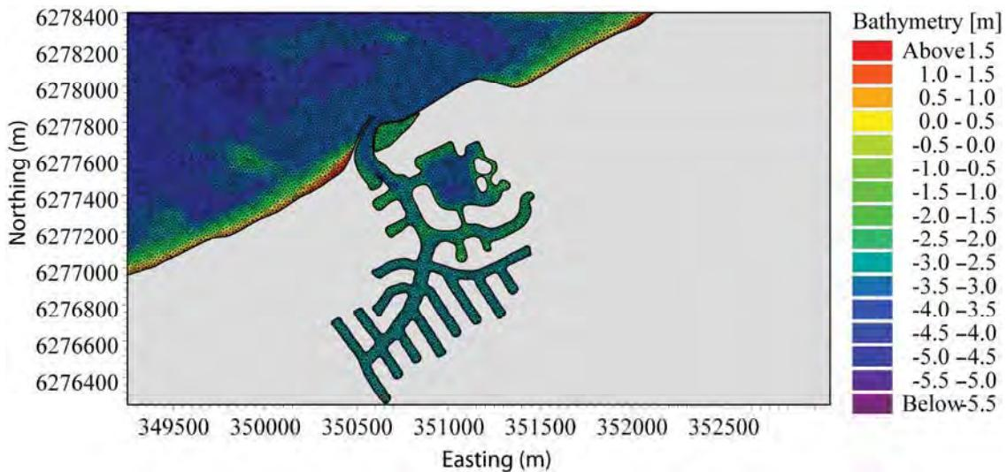
**Figure 4.78 Mesh grid and initial bathymetry in the vicinity of Port Geographe for Scenario 7 including proposed lagoon and all inner canal segments.**
