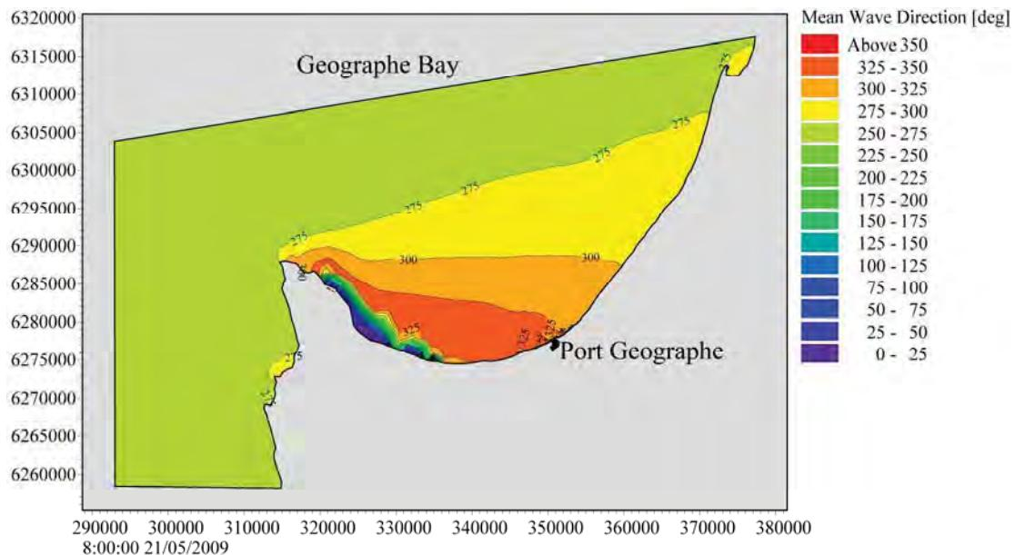
**Figure 3.6 Model-predicted mean wave direction showing wave refraction at Cape Naturaliste during typical southwest storms (on 21 May 2009).**
