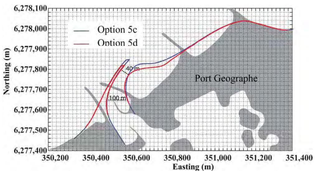
**Figure 4.61 Layout for Scenario 5 at Port Geographe. Blue line shows Scenario 4 - layout and the red line shows the layout for Scenario 5.**
