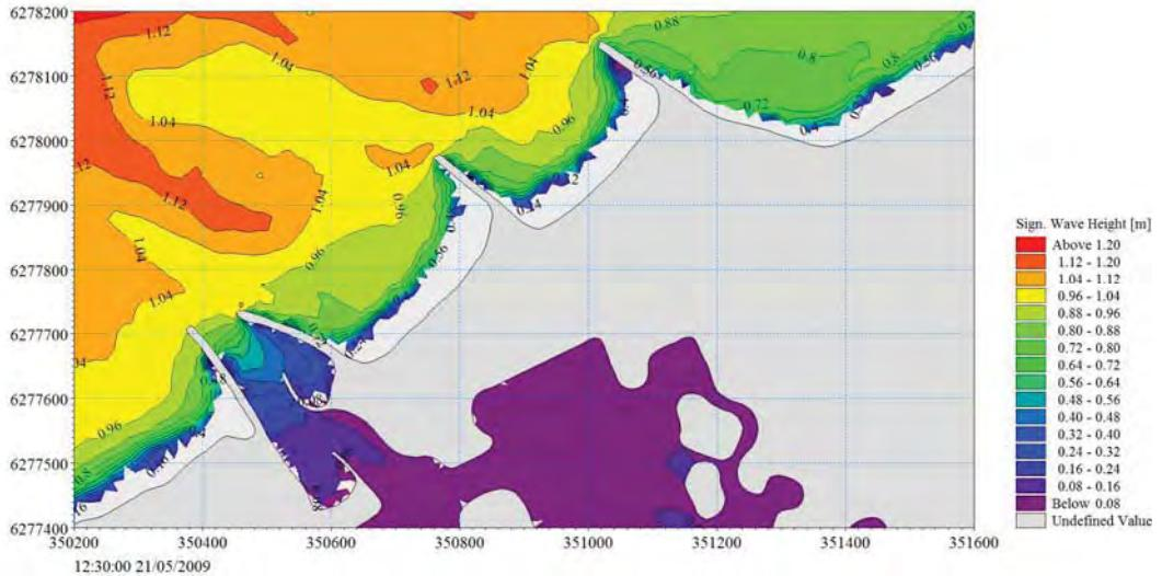
**Figure 4.103 Snapshot of predicted significant wave height in the Port Geographe area at the peak of storm on May 21 2009 for the existing groyne configuration.**
