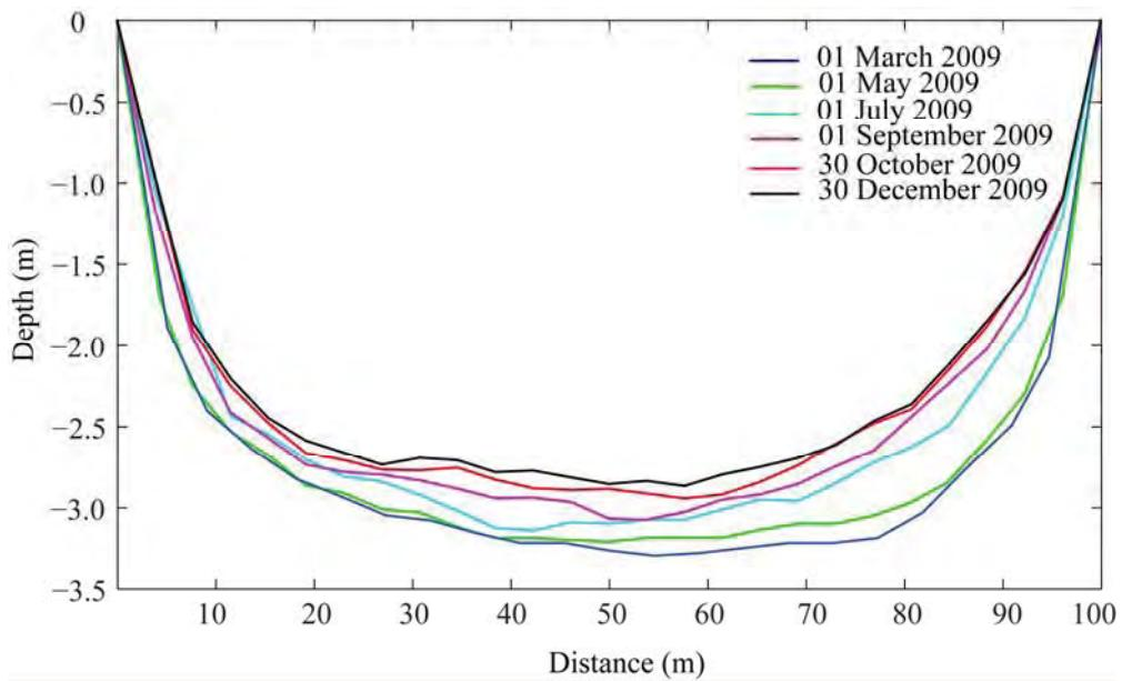
**Figure 4.80 Predicted bed levels across the harbour entrance channel (section x-y) of Port Geographe for Scenario 7 from 1 March to 30 December 2009.**
