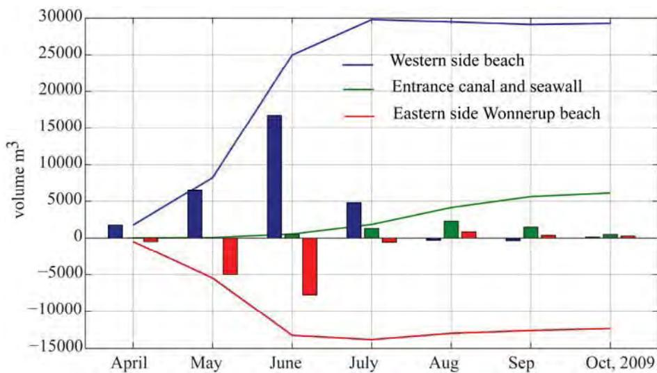
**Figure 4.57 Model-simulated monthly sand accretion and cumulative volume from 1 March to 30 October 2009 at different locations of Port Geographe for Scenario 4.**
