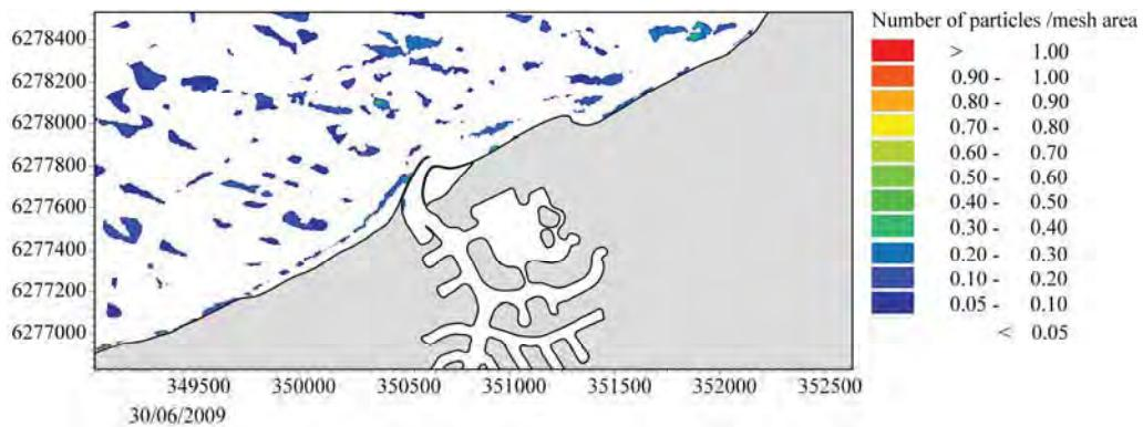
**Figure 4.90 Particle distribution in the vicinity of Port Geographe on 30 June 2009 for Scenario 8.**
