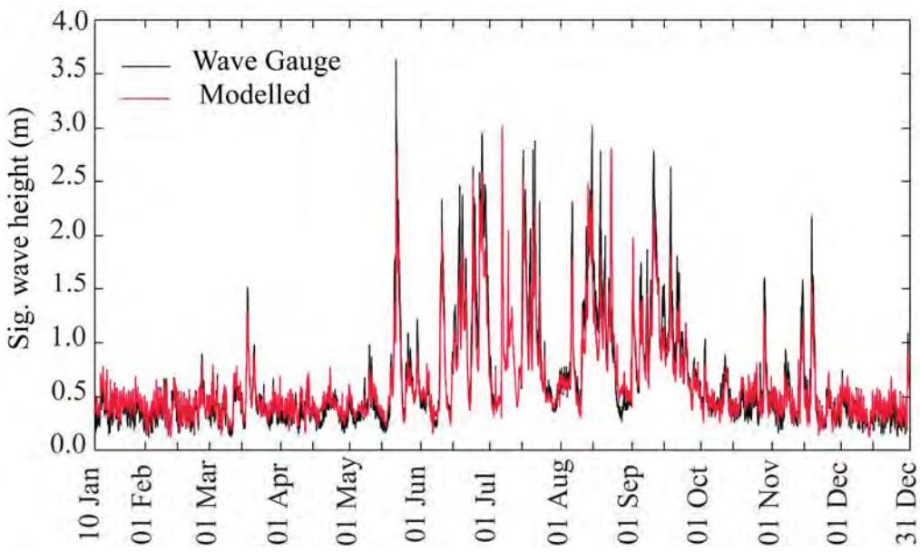
**Figure 3.7 Measured and predicted significant wave height at the AWAC site in 2009.**
