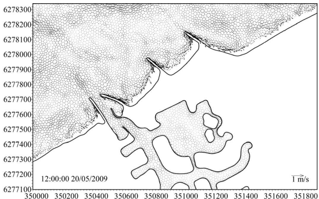
**Figure 4.9 Predicted velocity vectors in the vicinity of Port Geographe at the beginning of storm event (1200 hrs, 20 May 2009).**
