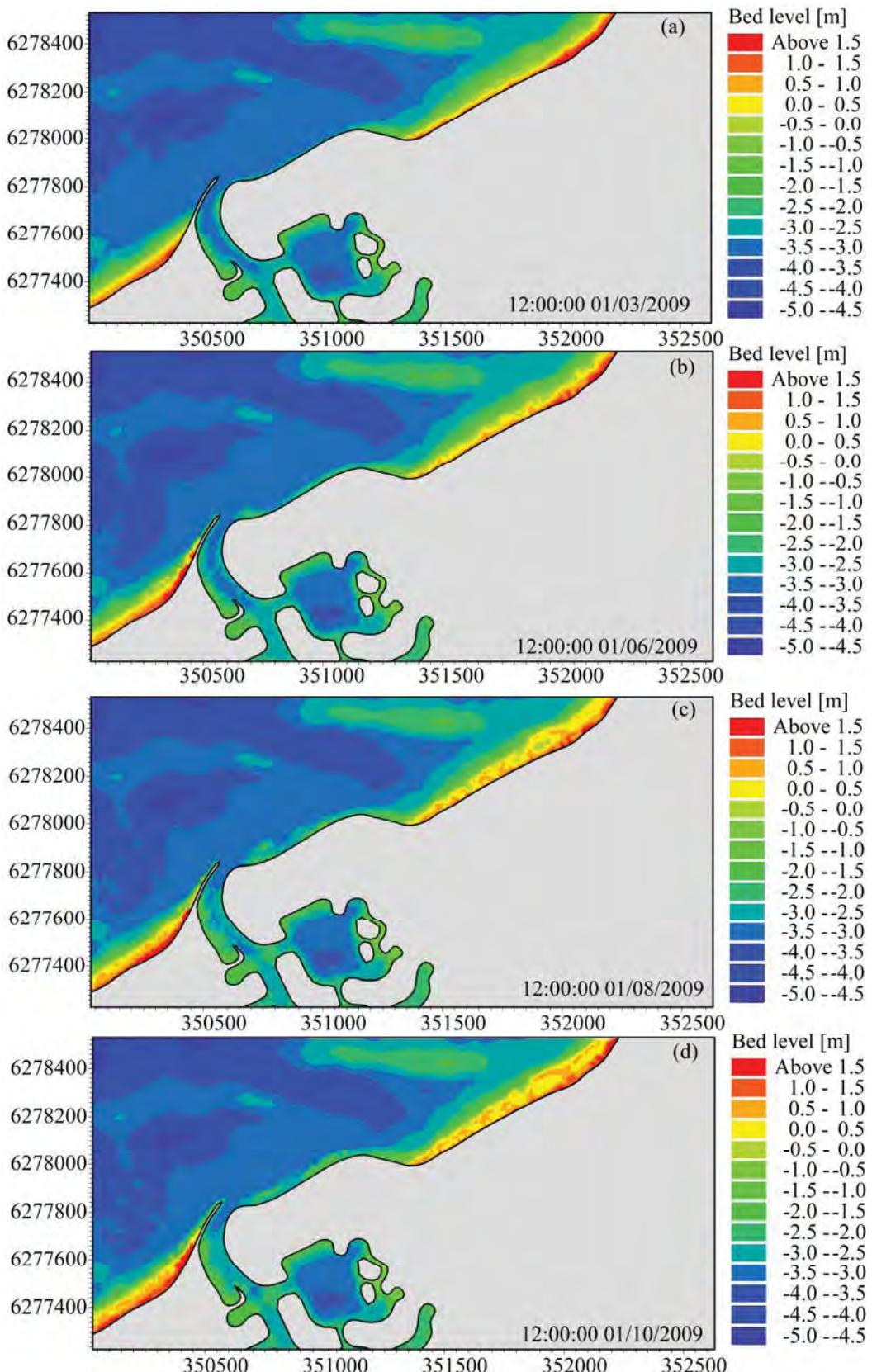
**Figure 4.47 Model-predicted bed levels in the vicinity of Port Geographe for Scenario 3 on 1 June 2009. (a) Model initial bathymetry on 1 March 2009; Predicted bed levels on: (b) 1 June 2009; (c) 1 August 2009; and, (d) 1 October 2009.**
