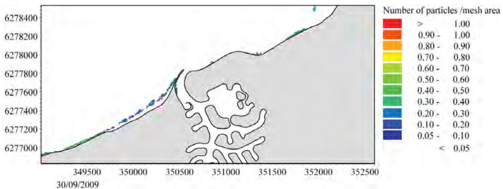
**Figure 4.51 Particle distribution in the vicinity of Port Geographe on 30 September 2009 for Scenario 3.**
