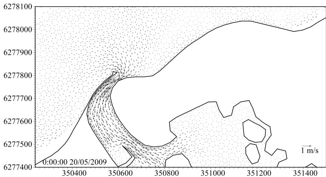
**Figure 4.28** Model-predicted current pattern in the vicinity of Port Geographe for Scenario 2 (Option 5a) prior to storm event (0000 hr, 20 May 2009).
