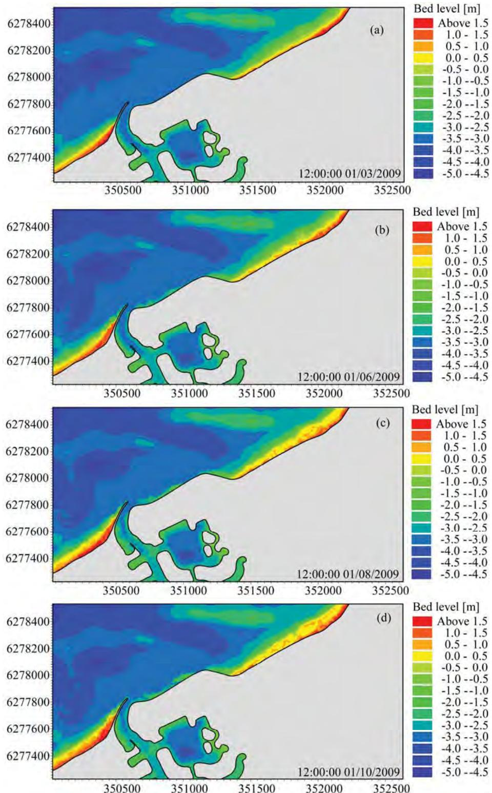
**Figure 4.71 Model-predicted bed levels in the vicinity of Port Geographe for Scenario 6.**
