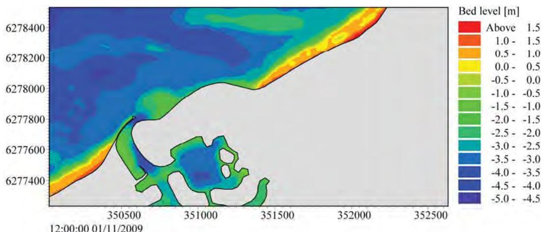
**Figure 4.36 Model-predicted bed levels in the vicinity of Port Geographe for Scenario 2 on 01 November 2009.**
