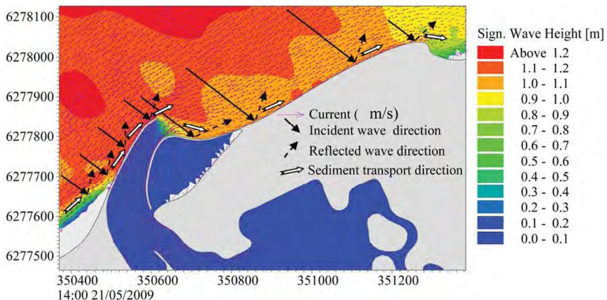
**Figure 4.108 Schematic of typical wave condition, easterly currents during storm conditions on 21st May 2009 for Scenario 8.**
