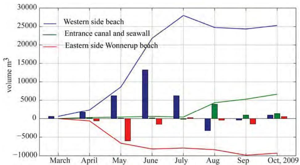
**Figure 4.49** Model-simulated monthly sand accretion and cumulative volume during 1 March to 30 October 2009 in different locations of Port Geographe for Scenario 3.
