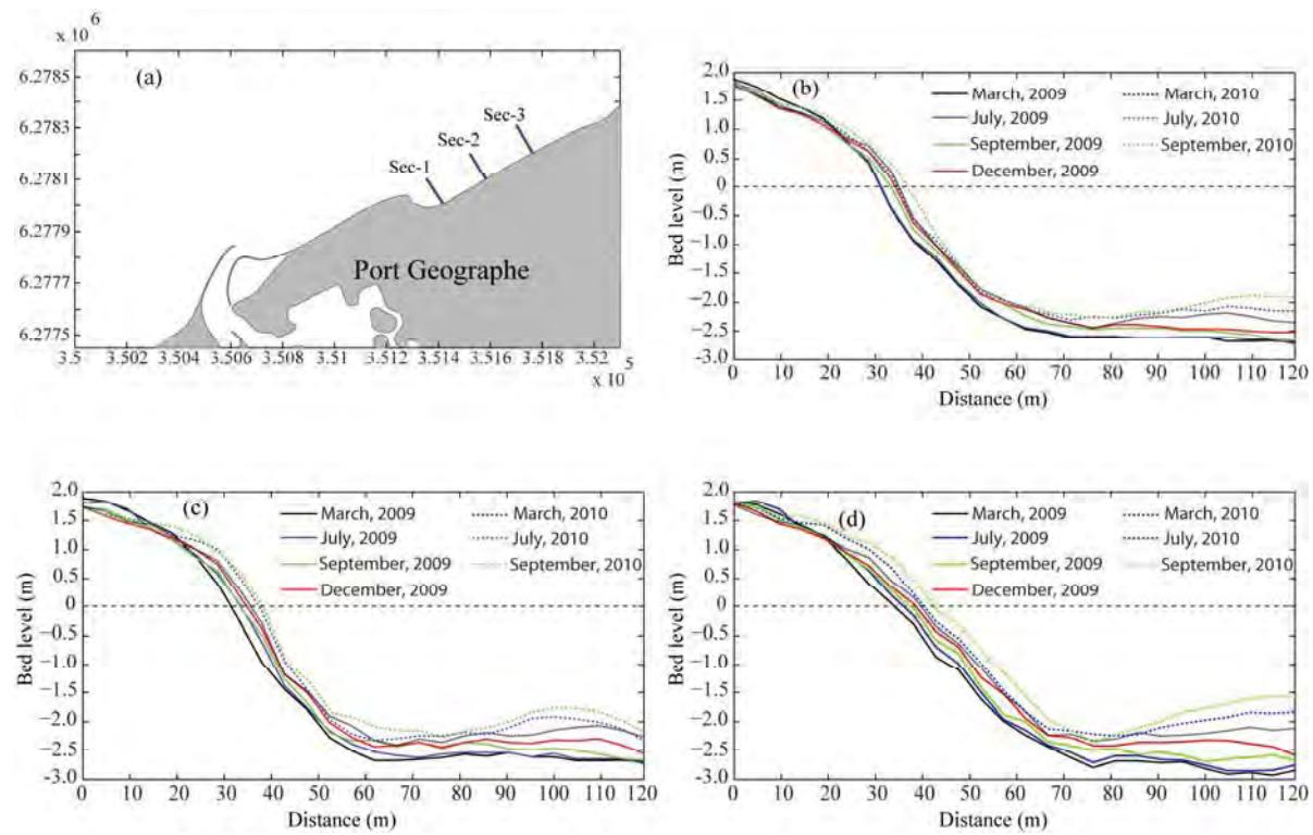
**Figure 4.99 Predicted beach profiles in 2009 and 2010 along Wonnerup Beach for Scenario 8. (a) location of cross-sections and predicted profiles for: (b) section 1 (Sec-1); (c) section 2 (Sec-2); and; (d) section 3 (Sec-3).**
