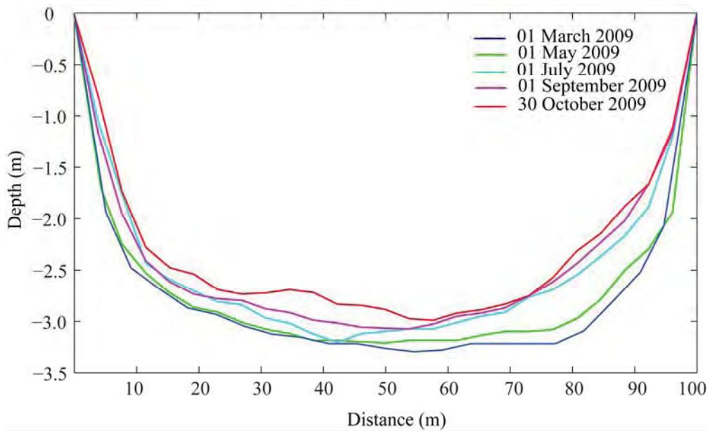
**Figure 4.48** Model-predicted bed levels across the harbour entrance channel (Cross-section x-y) of Port Geographe for Scenario 3 during 1 March to 30 October 2009.
