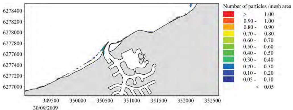
**Figure 4.83 Particle distribution in the vicinity of Port Geographe on 30 September 2009 for Scenario 7.**
