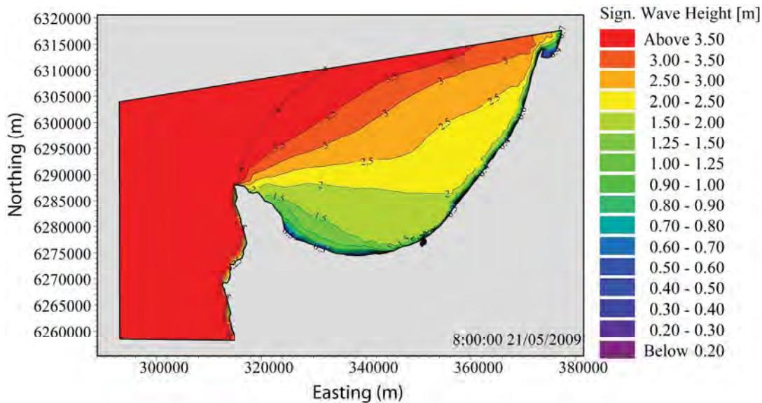
**Figure 4.13 Snapshot of model-predicted wave height distribution during a storm event (on 21 May 2009).**
