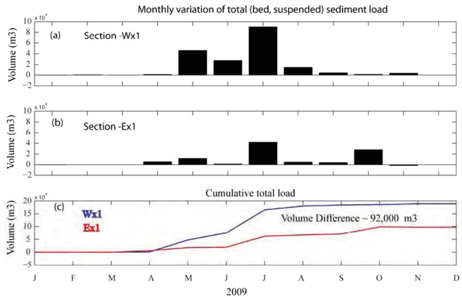
**Figure 4.23 Predicted total sediment load transport. (a) monthly variation of total load through western section; (b) monthly variation transport through eastern section; and, (c) cumulative load through western (blue line) and eastern sections (red line)**
