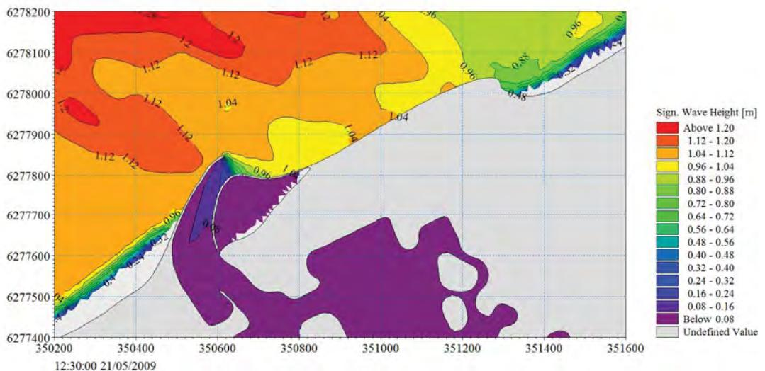
**Figure 4.104 Snapshot of predicted significant wave height in the Port Geographe area at the peak of storm on May 21 2009 for the existing groyne configuration.**
