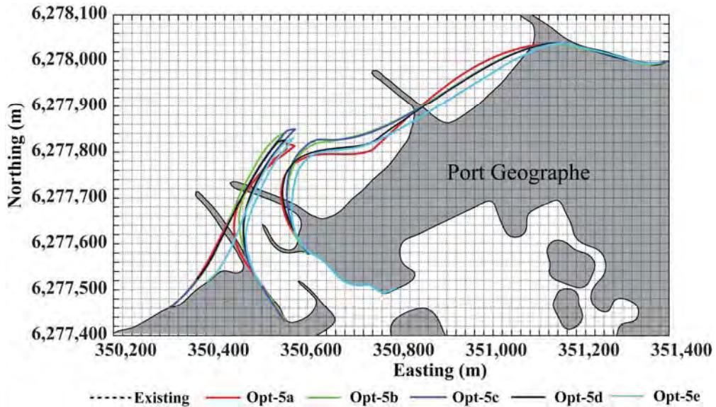
**Figure 4.1:** Layouts for scenarios 2 to 6, which examined different alignments of the western breakwater, harbour entrance channel dimensions and alignment of the seawall to the east of the harbour entrance.
