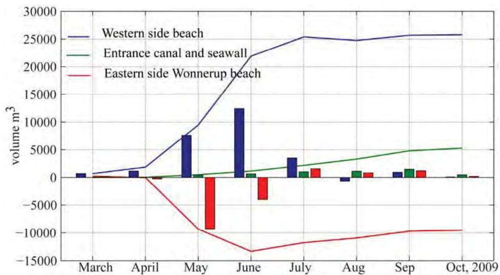
**Figure 4.65 Model-simulated monthly sand accretion and cumulative volume during 01 March to 30 October 2009 at different locations of Port Geographe for Scenario 5.**
