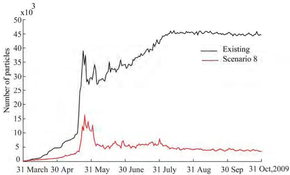
**Figure 4.92 Predicted cumulative number of particle (seagrass wrack) at the western beach, Port Geographe from March to October 2009 for Scenario 8.**
