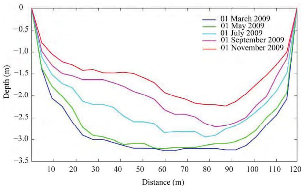
**Figure 4.38 Predicted bed levels (in AHD) across the harbour entrance channel (Section x-y) of Port Geographe for Scenario 2 during March to November 2009.**
