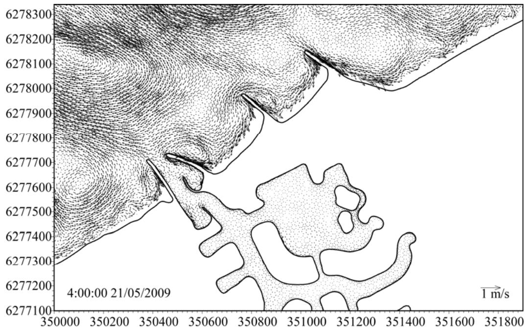
**Figure 4.10 Predicted velocity vectors in the vicinity of Port Geographe during storm event (0400 hrs, 21 May 2009).**
