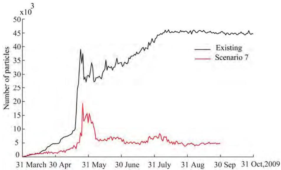
**Figure 4.84 Predicted cumulative number of particle (seagrass wrack) at the western beach, Port Geographe from March to October 2009 for Scenario 7.**
