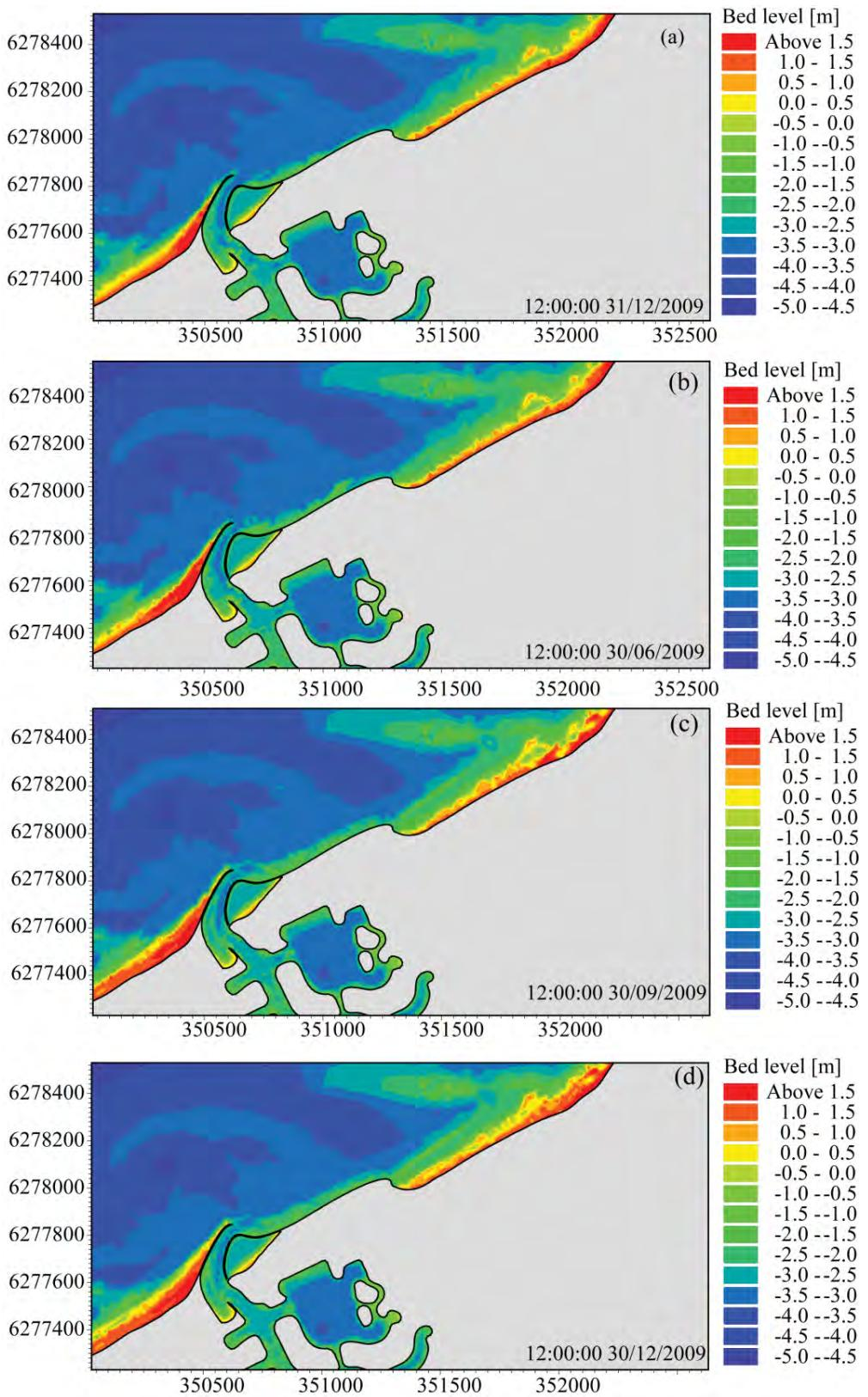
**Figure 4.93 Model-predicted bed levels in the vicinity of Port Geographe for scenario 8 with initial saturated beach on the western side of Port Geographe. (a) Model initial bathymetry on 31 Dec 2009, and predicted bed levels on (b) 30 June 2009; (c) 30 September 2009; and, (d) 30 December 2009**
