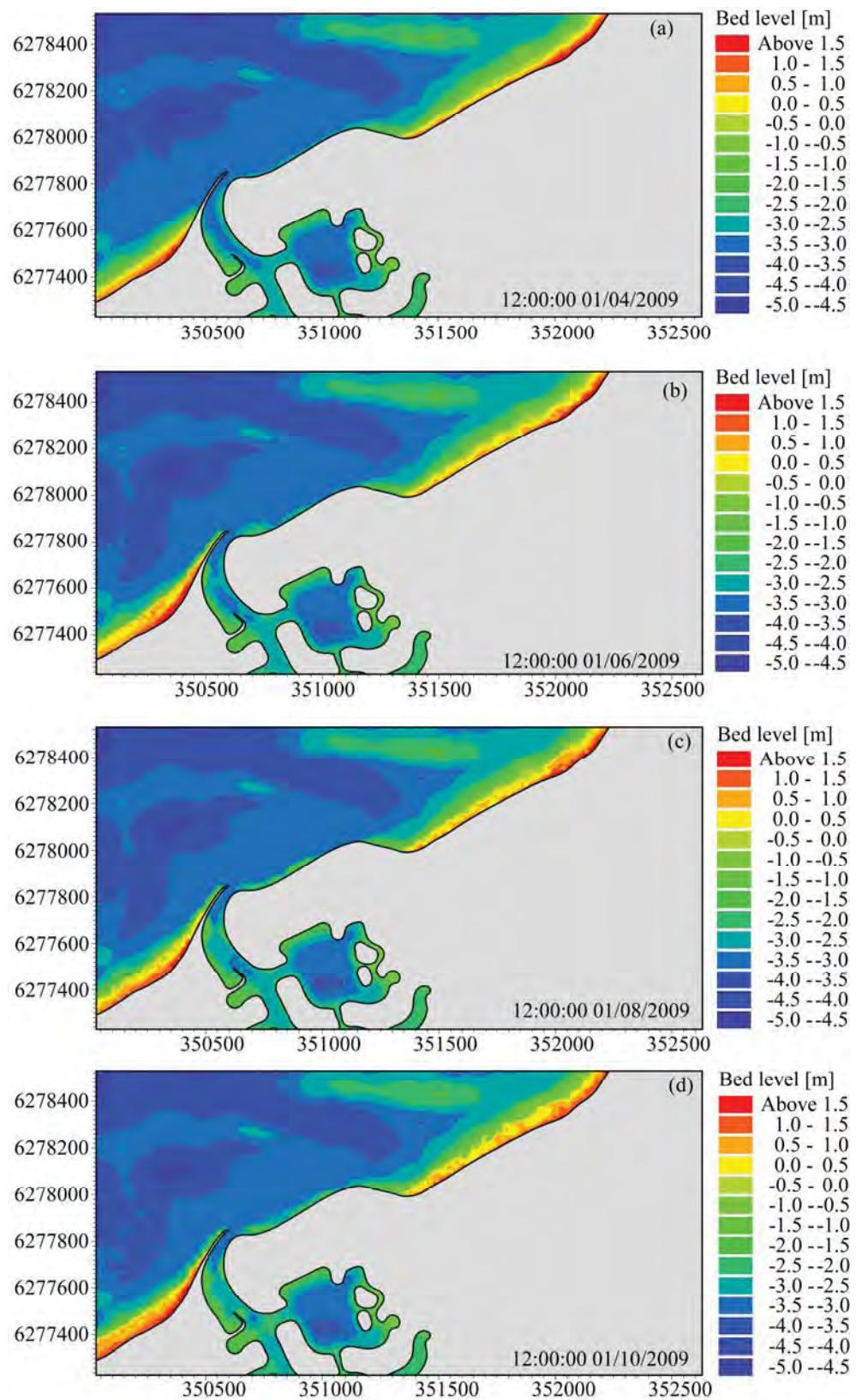
**Figure 4.55 Model-predicted bed levels in the vicinity of Port Geographe for Scenario 4. (a) Model initial bathymetry on 01 April 2009 and predicted bed levels on: (b) 01 June 2009; (c) 01 August 2009; and, (d) 01 October 2009.**
