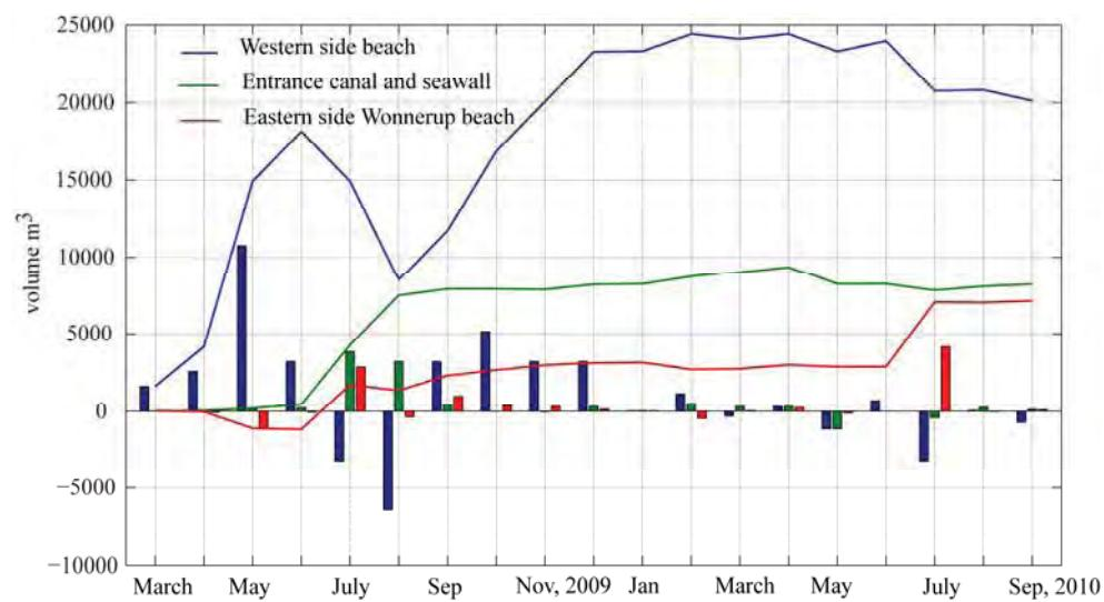
**Figure 4.98 Model-simulated monthly sand accretion and cumulative volume during 01 March 2009 to 30 September 2010 at different parts of Port Geographe for scenario 8.**
