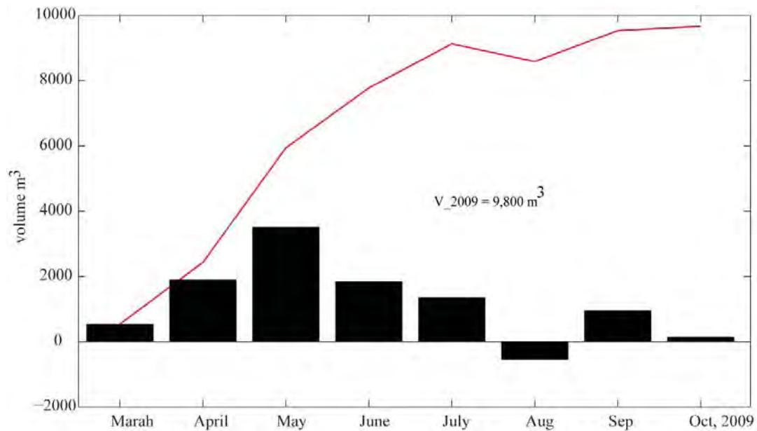
**Figure 4.39** Predicted monthly sand accretion and cumulative sand volume from 1 March to 1 November 2009 along the western beach (see Figure 4.37 for selected area) under Scenario 2.
