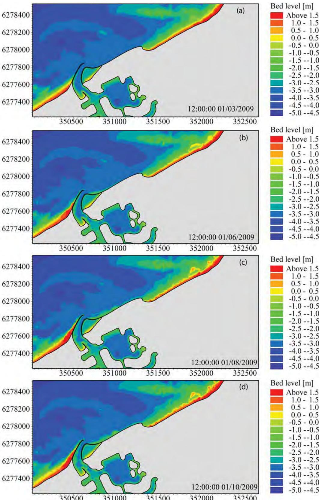
**Figure 4.87 Model-predicted bed levels in the vicinity of Port Geographe for Scenario 8.(a) Model initial bathymetry on 01 March 2009, and predicted bed levels on (b) 1 June 2009; (c) 01 August 2009; and, (d) 01 October 2009.**
