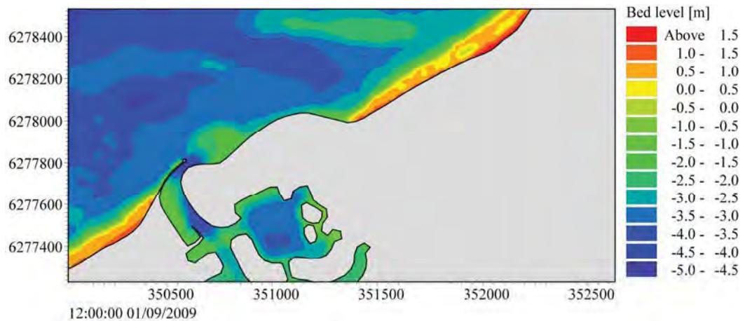
**Figure 4.35 Model-predicted bed levels in the vicinity of Port Geographe for Scenario 2 on 01 September 2009.**
