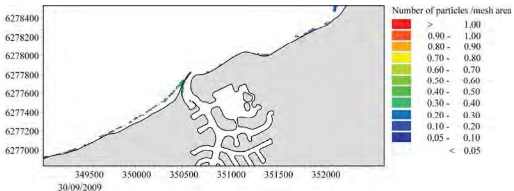
**Figure 4.75 Particle distribution in the vicinity of Port Geographe on 30 September 2009 for Scenario 6.**
