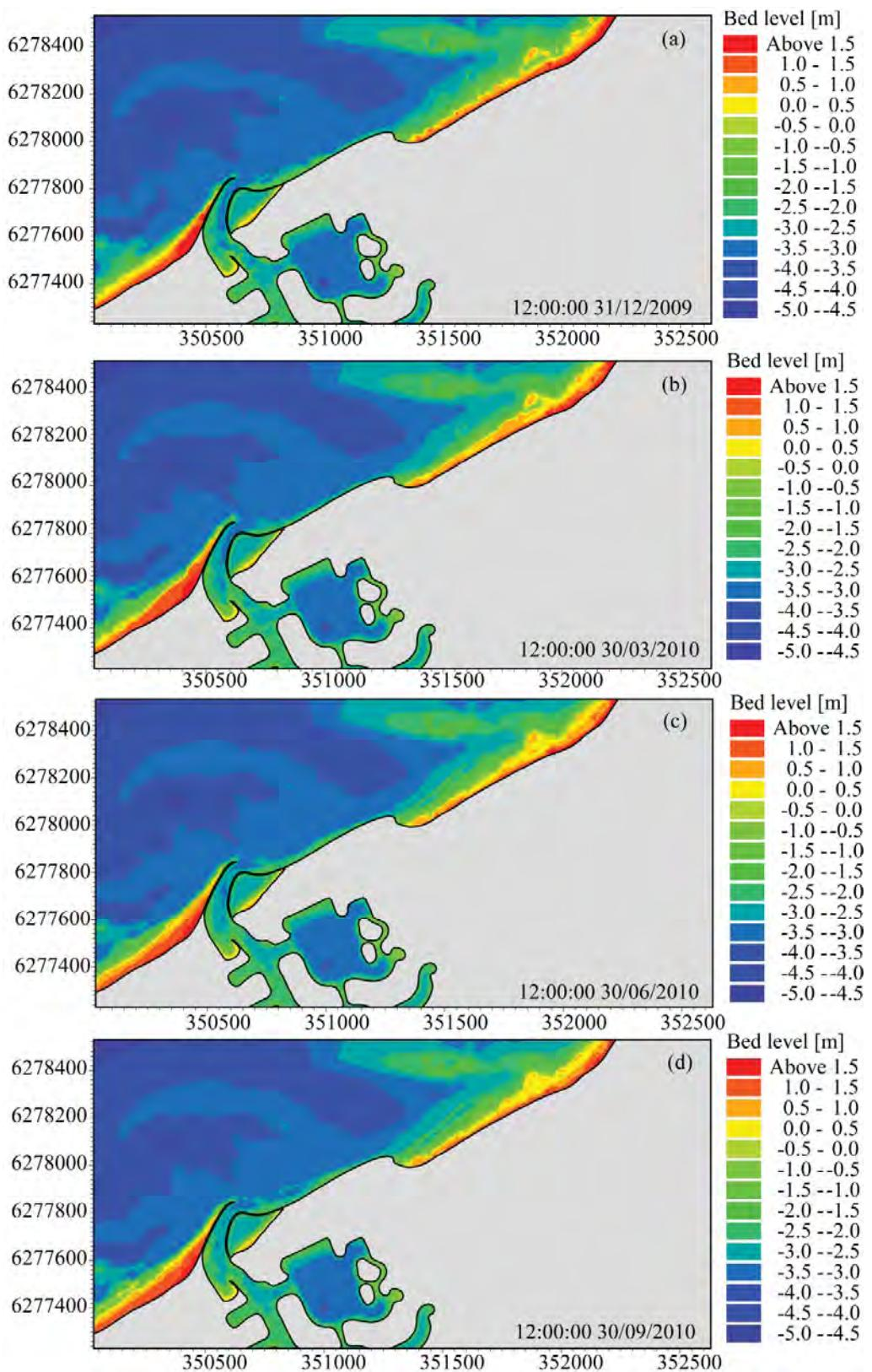
**Figure 4.96 Model-predicted bed levels in the vicinity of Port Geographe for scenario 8 for 2010 with initial saturated beach on the western side of Port Geographe. (a) Model initial bathymetry on 31 Dec 2009 and predicted bed levels on (b) 30 March 2010; (c) 30 June 2010; and, (d) 30 September 2010,**
