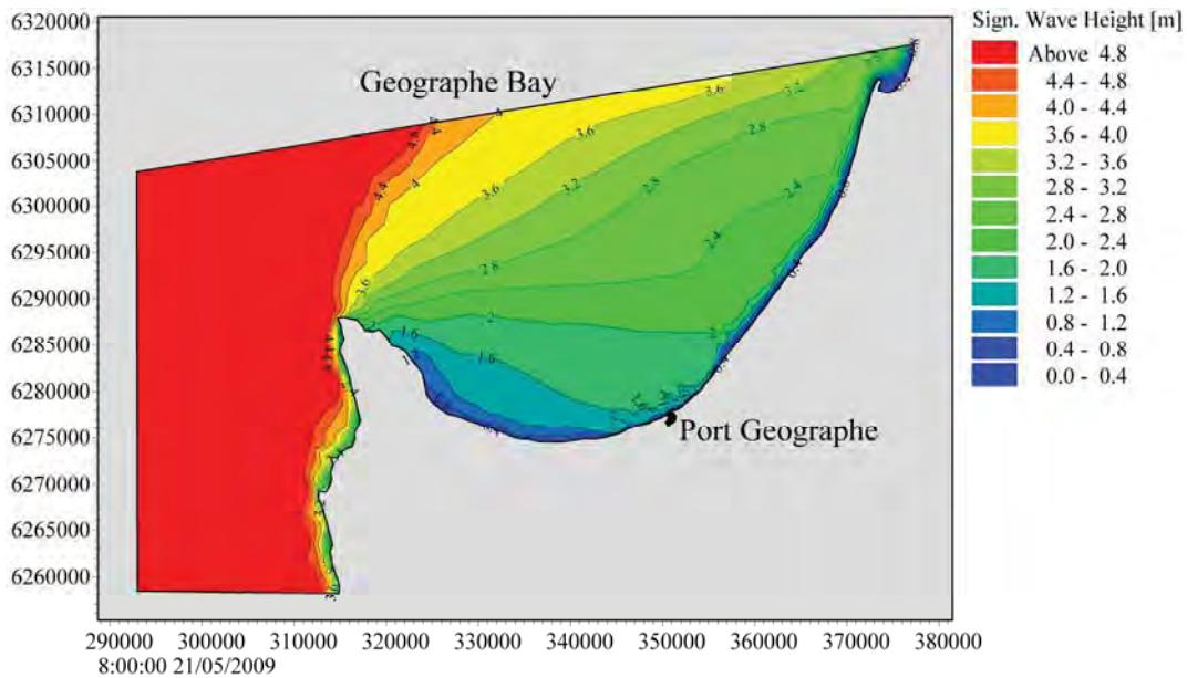
**Figure 3.5 Model-predicted wave height distribution showing wave refraction at Cape Naturaliste during typical southwest storms (on 21 May 2009).**
