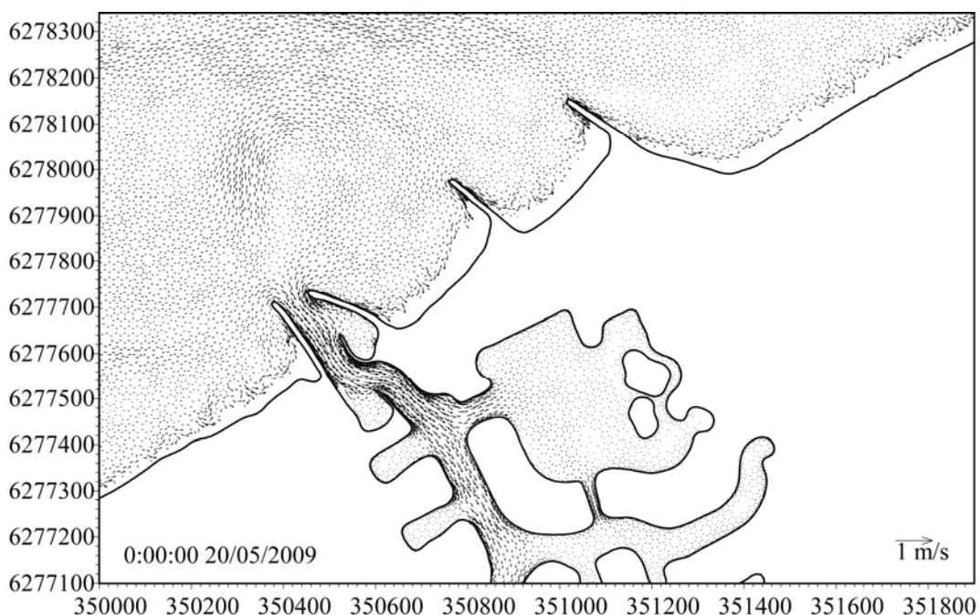
**Figure 4.8 Predicted velocity vectors in the vicinity of Port Geographe prior to storm event (0000 hrs, 20 May 2009).**
