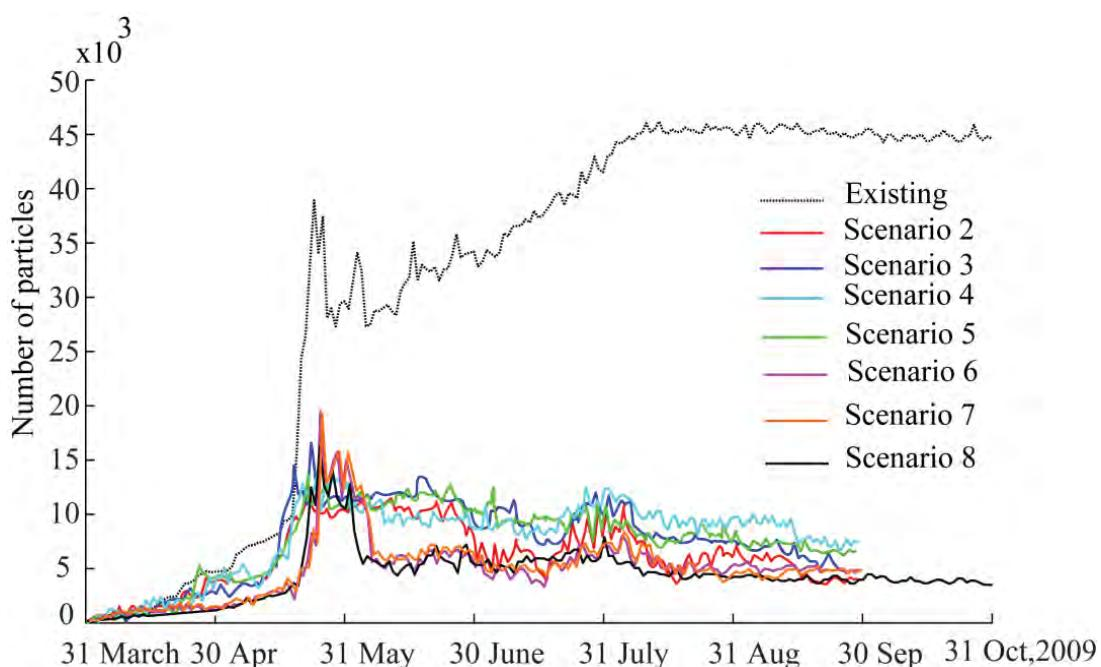
**Figure 4.106 Comparison predicted cumulative number of particles (seagrass wrack) at the western beach, Port Geographe for 2009 for the different layouts (Scenarios 1- 8)**
