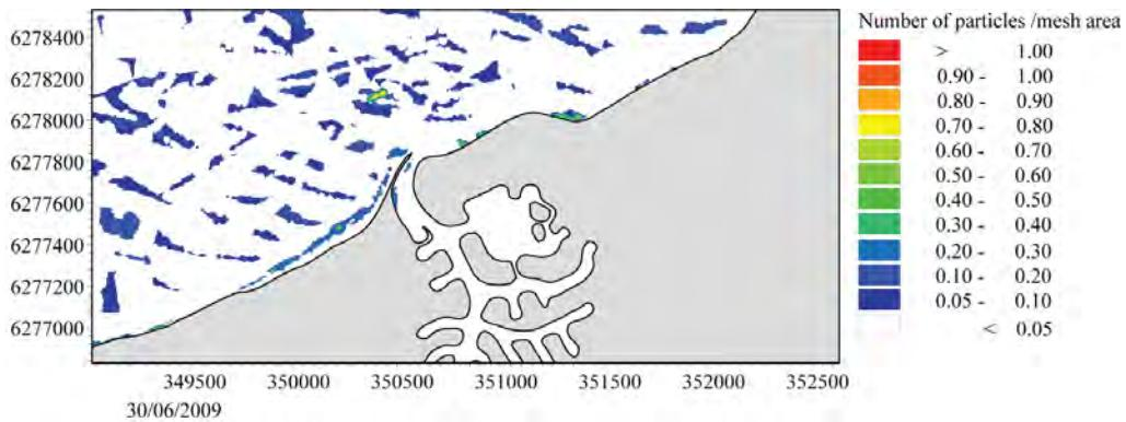
**Figure 4.50 Particle distribution in the vicinity of Port Geographe on 30 June 2009 for Scenario 3.**
