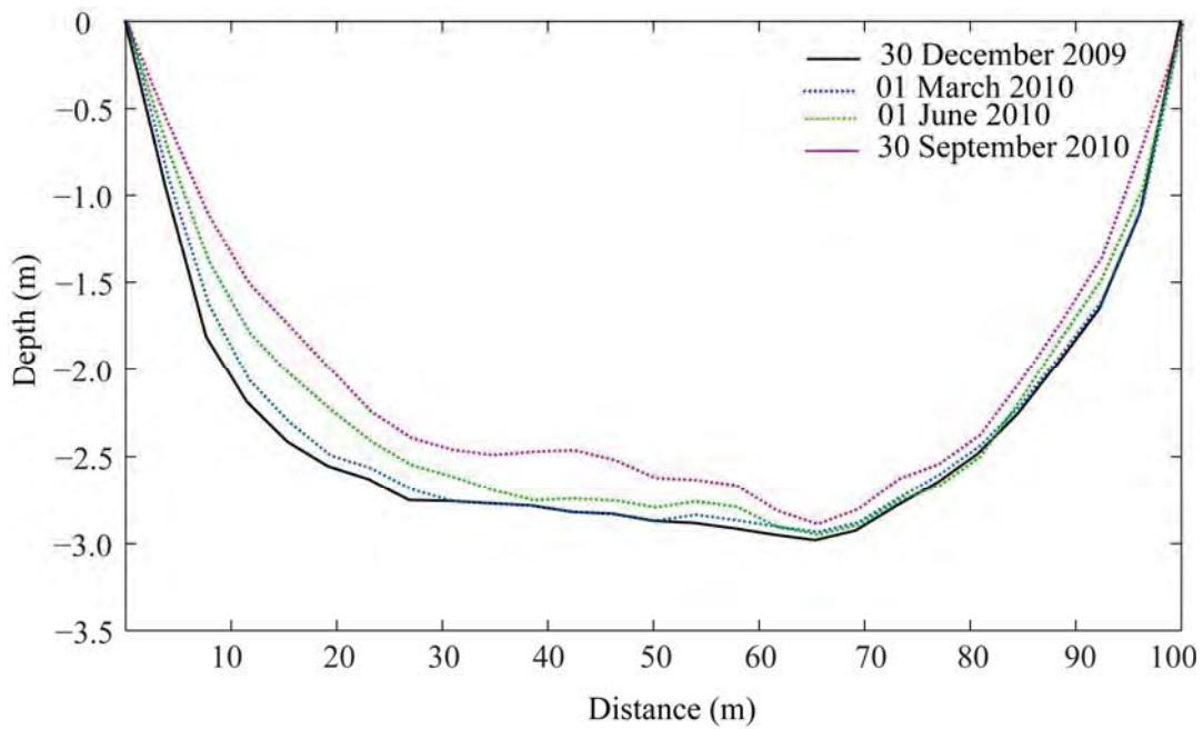
**Figure 4.97 Model-predicted bed levels across the entrance canal (section x-y) of Port Geographe for scenario 8 during 01 March to 30 September 2010.**
