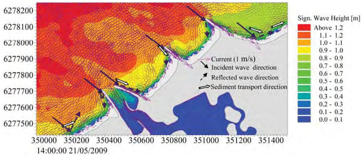
**Figure 4.107 Schematic of typical wave conditions, easterly currents during storm conditions on 21st May 2009 for existing configuration.**
