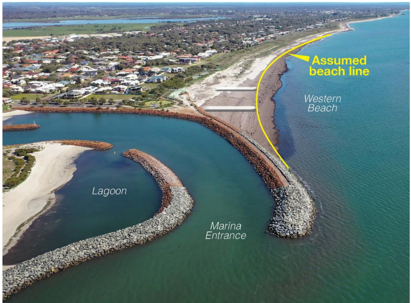
Figure 19: Western Beach 4 – Right-Angle Low-Profile Sand Bag Groynes
