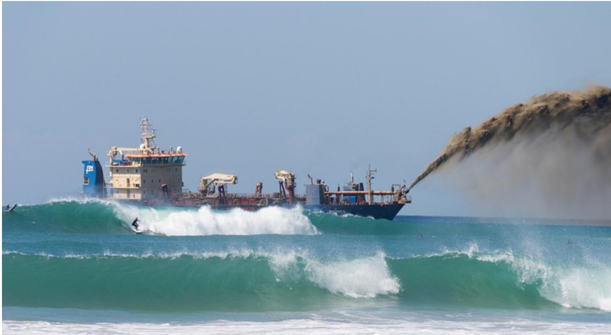
Figure 37: Example of a Trailing Suction Hopper Dredge “rainbowing” material for beach nourishment in Queensland
