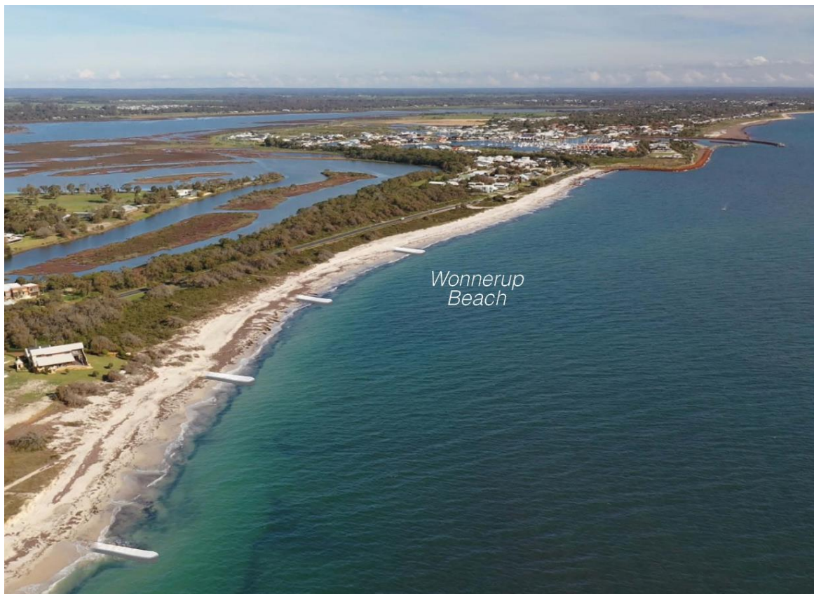
Figure 38: Idea Wonnerup 10 - Aerial photo showing newly constructed sand bag groynes at East Wonnerup
