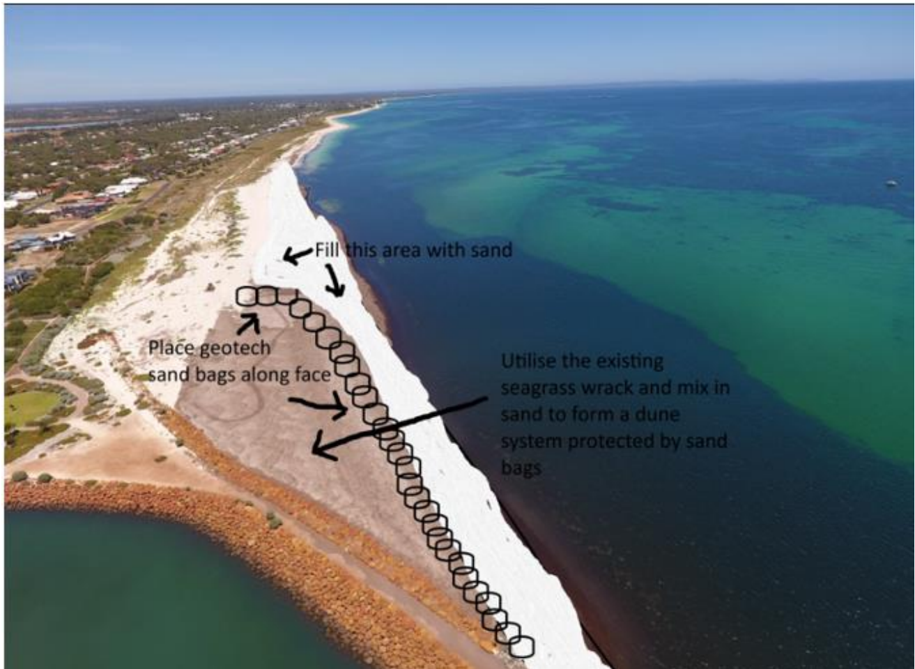
Figure 23: Idea Western Beach 8 – Build a beach profile with sandbags (community submission)
