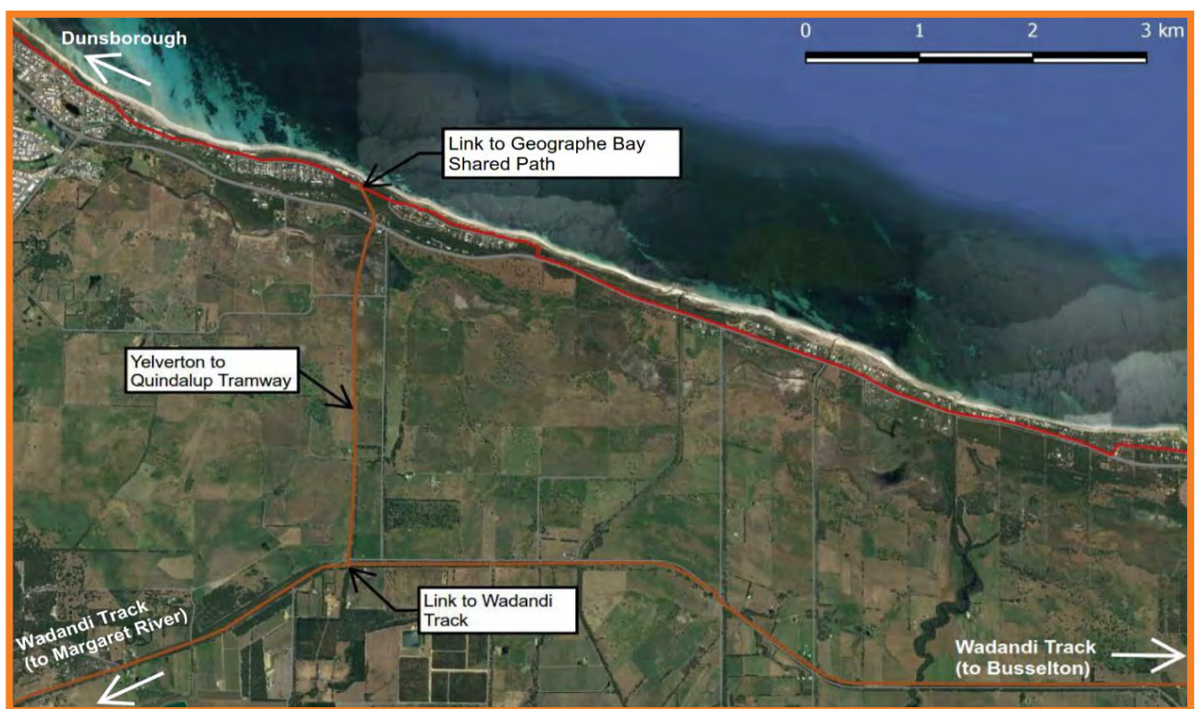
Figure 4.7 The Yelverton-Quindalup tramway formation could be used to provide an important connection between the Wadandi Track and the Geographe Bay Shared Path.
