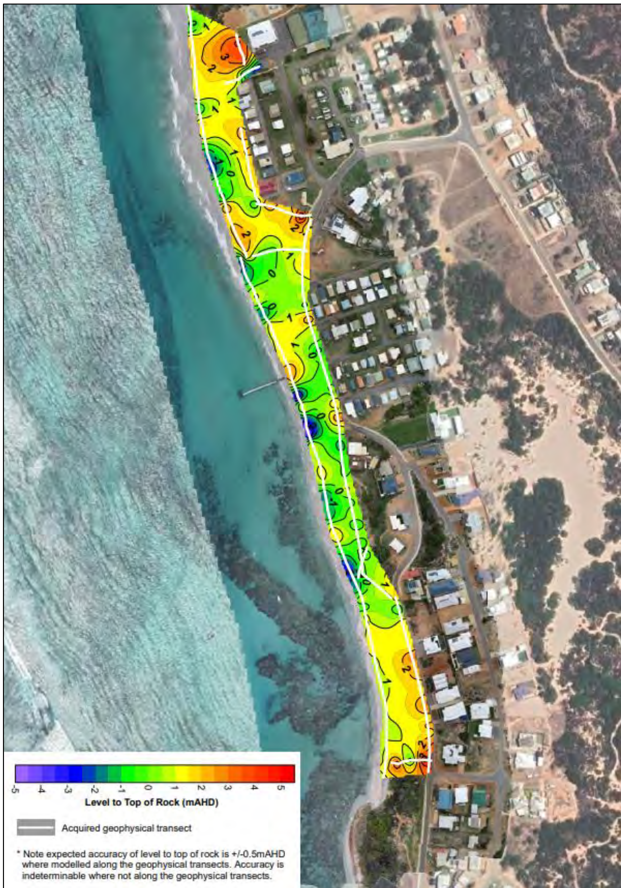
Figure 18: Interpreted level to top of rock (mAHD) from Northampton geotechnical investigation; it is possible that Glance Cove is protected from chronic erosion hazards by natural underlying rock.
