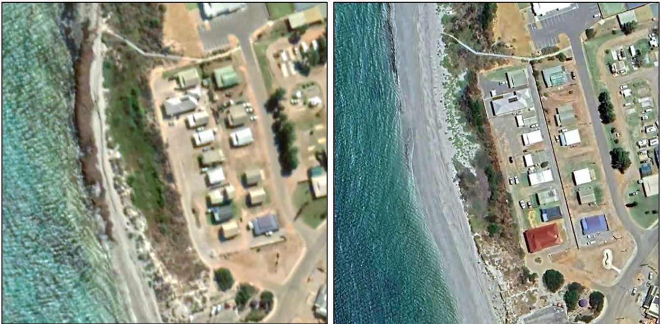
Figure 17: Glance Cove at Horrocks hotspot, showing pre-relocation of front property access in 2019 (left) and post-relocation in 2023 (right). Also visible in the 2023 image is the appearance of a defined erosion scarp plus lost dune and vegetation.
