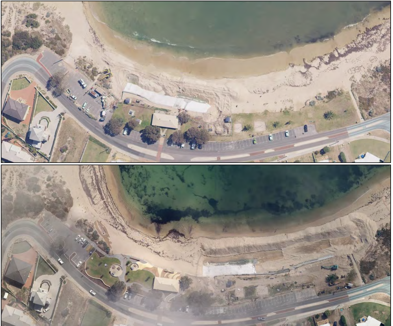
Figure 48: Construction of sheet piled seawall at Falcon Bay to Rakoa St hotspot, showing stage 1 in 2018 (top) and stage 2 in 2019 (bottom).
