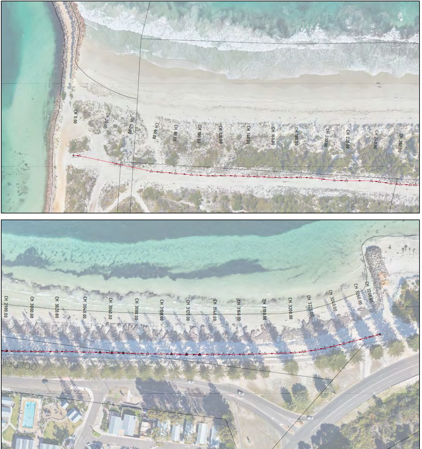
Figure 63: As-constructed survey of permanent pipe location at the northern terminus (top) and near the southern terminus (bottom). Not shown is an additional 300m of pipeline which continues beyond the groyne in the bottom image.
