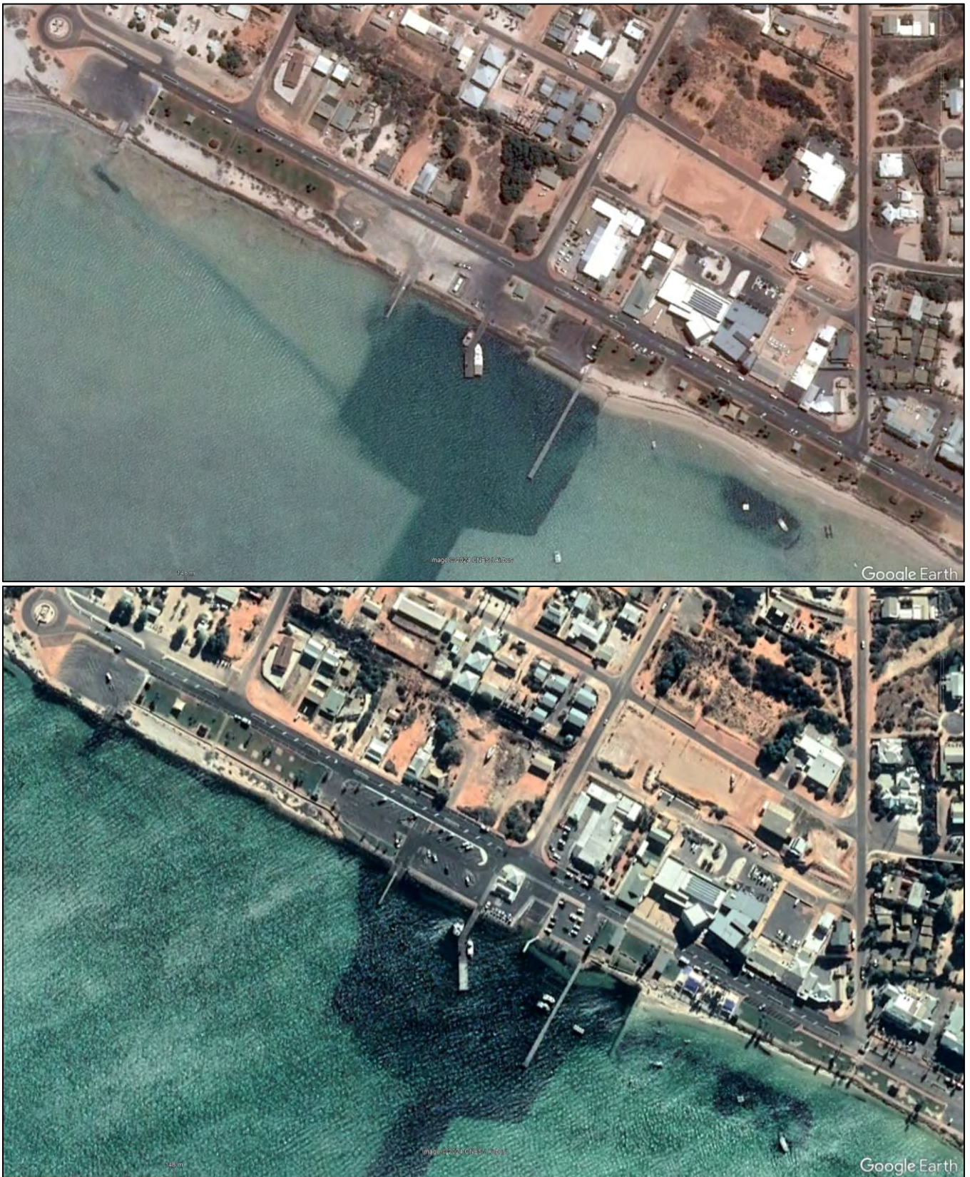
Figure 16: Denham pre-construction in 2015 (top) and 2018 (bottom); showing refurbished revetment at the marine facility foreshore and immediately northwest, plus the added sheet pile groyne immediately southeast of the jetties.
