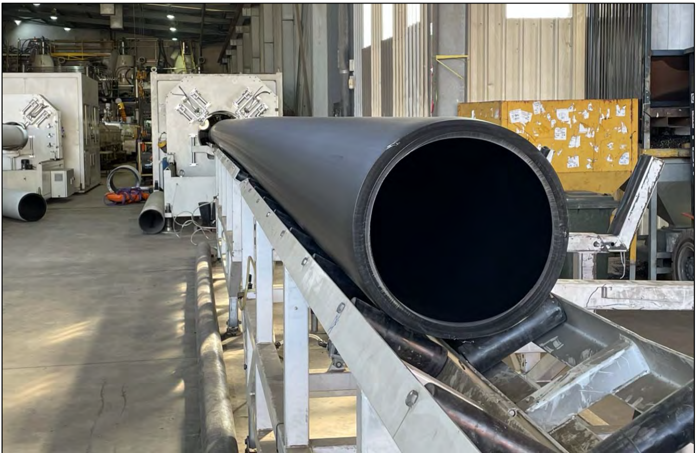
Figure 62: HDPE pipeline segment manufacturing at Acu-Tech, Perth in 2024.
