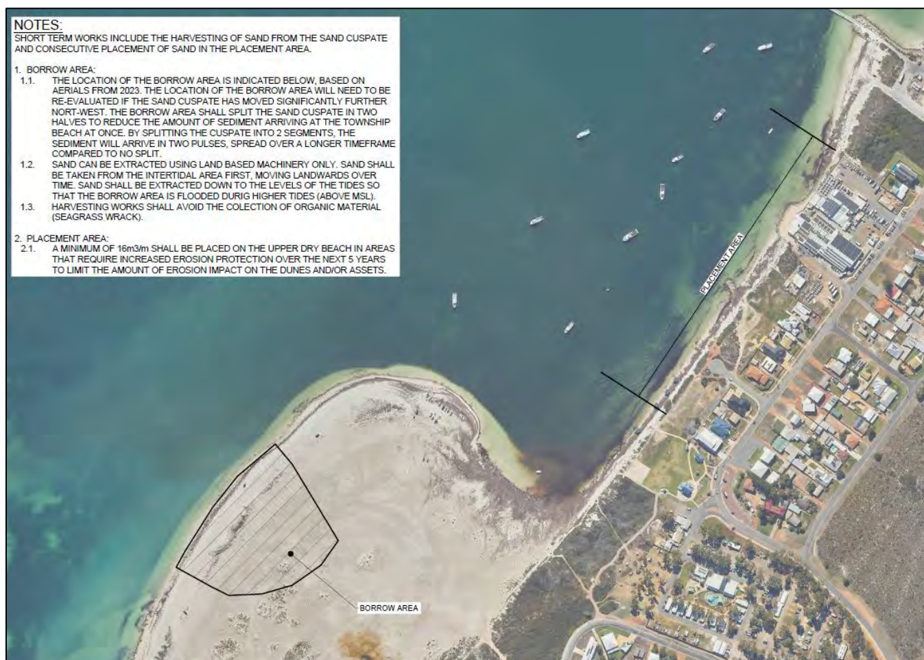
Figure 24: Preferred design for Cervantes erosion adaptation using sand from the cuspate foreland for nourishment along the hotspot extent (sourced from Water Technology 2024).
