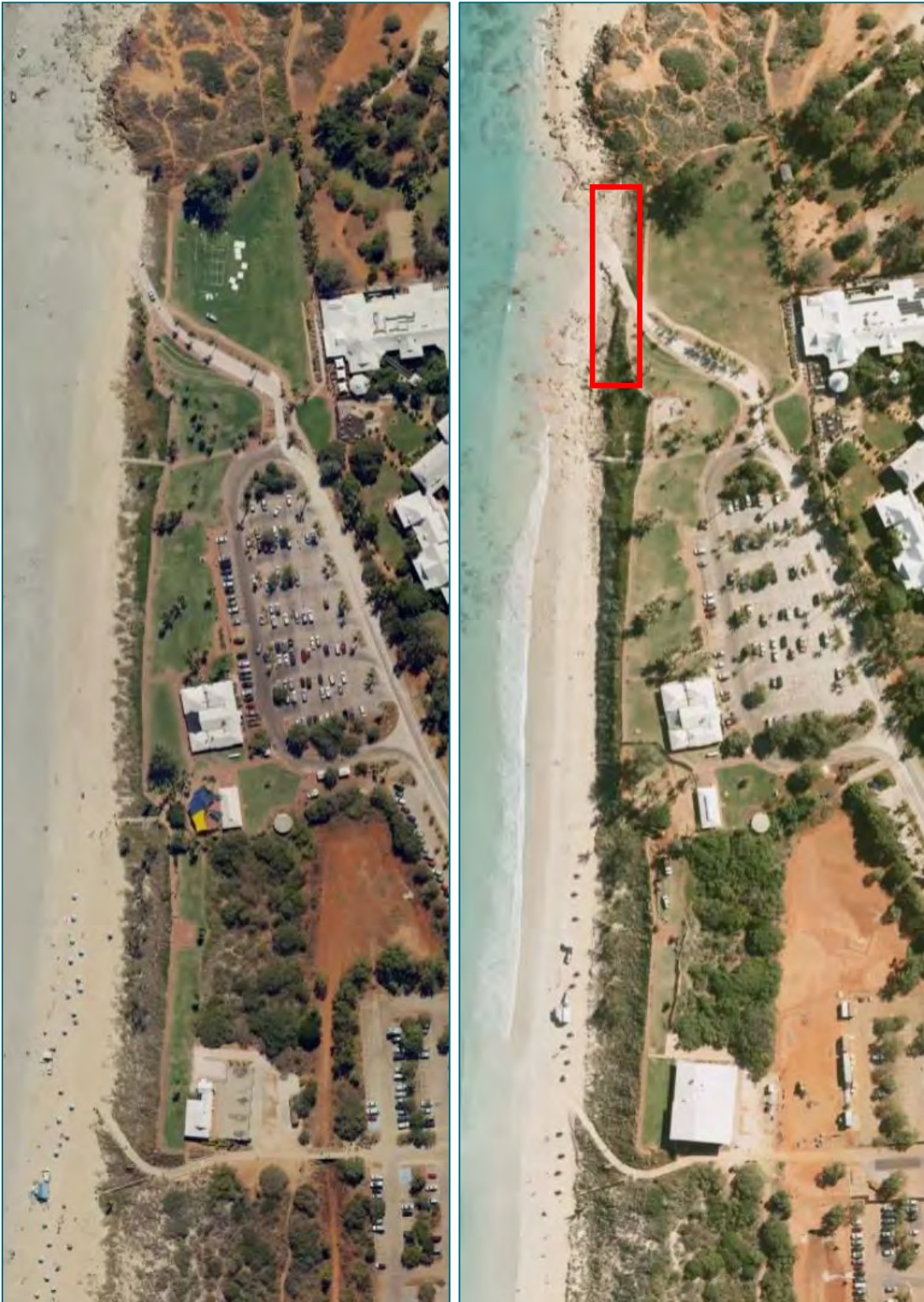
Figure 9: Cable Beach Foreshore nominated hotspot, showing 2017 (left) and 2024 (right). Erosion at the dune toe can be observed since 2017, particularly around beach access where the 2024/25 H-CAP revetment is planned (highlighted in red).
