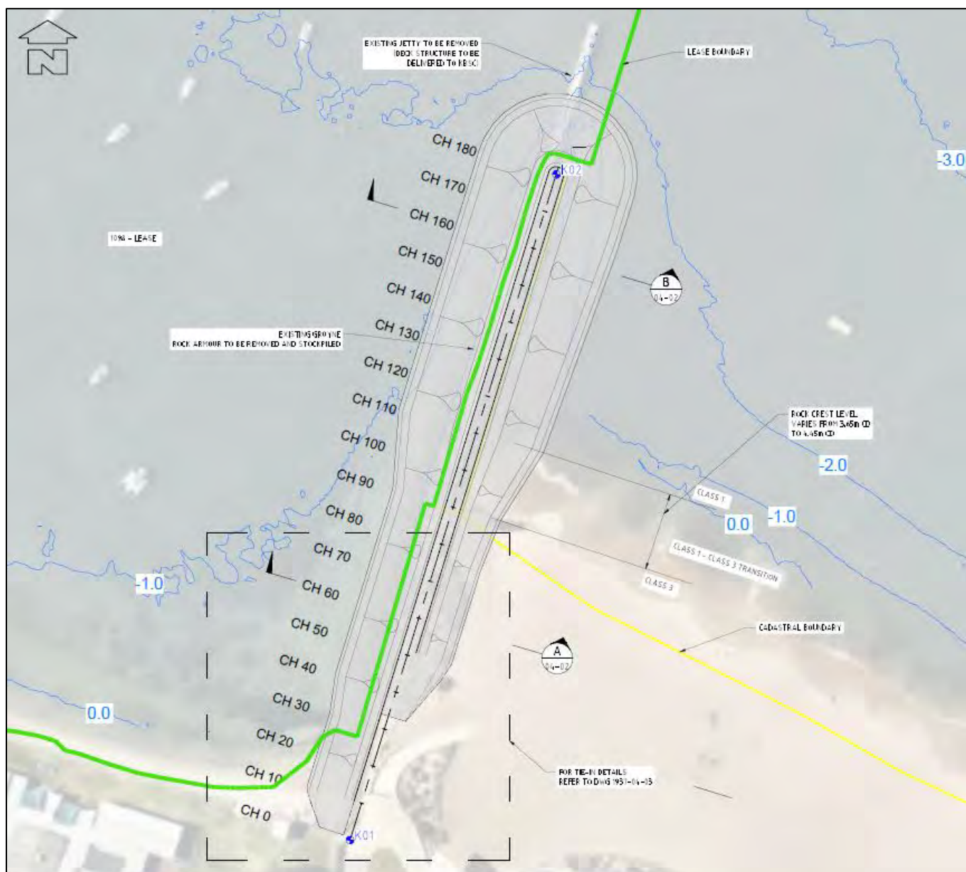
Figure 50: Notional plan of Koombana Bay western groyne upgrade and refurbishment by DoT and the City as part of Transforming Bunbury Waterfront Stage 3, co-funded by DRF in 2024/25. Note design of the groyne head is still under revision at the time of this review, to avoid impacting the adjacent jetty (sourced from Advisian 2024).
