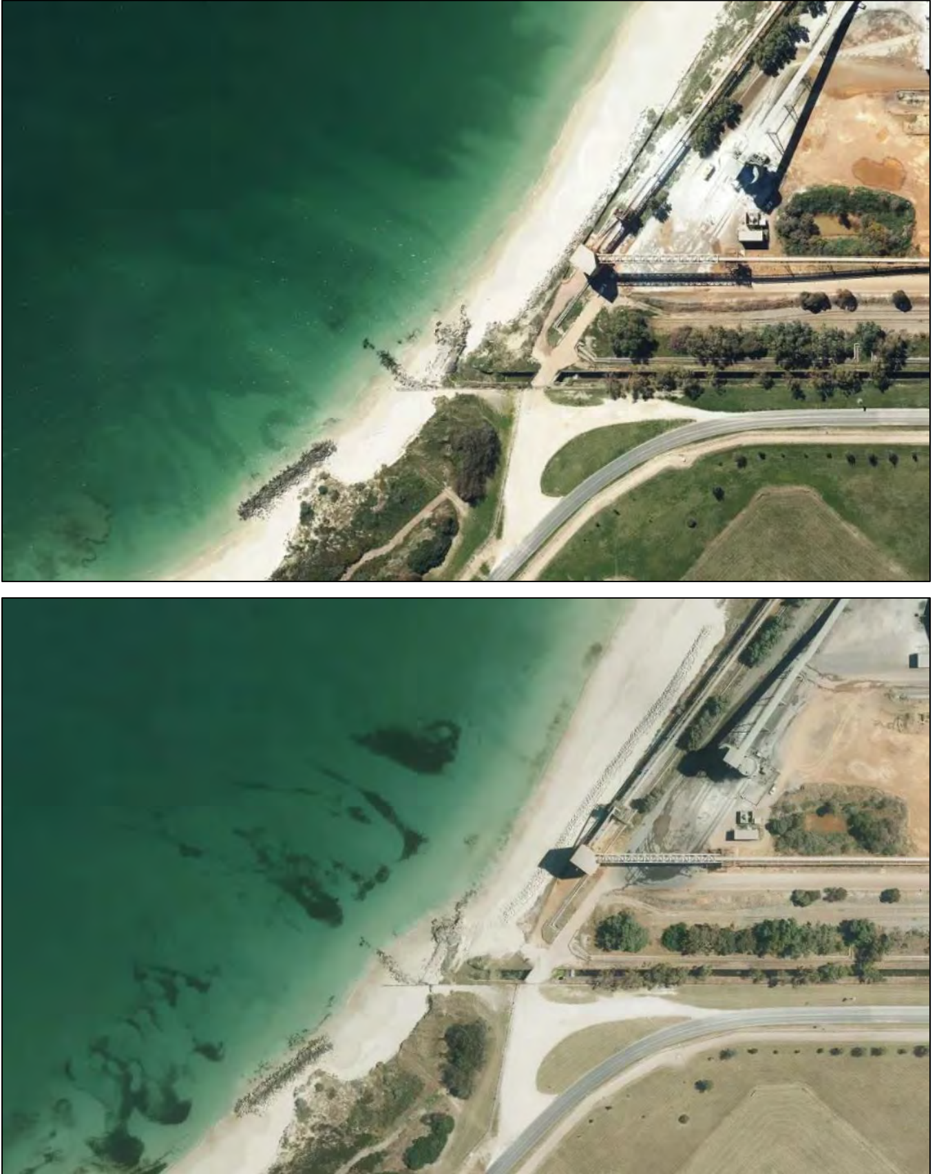
Figure 41: Formalised rock revetment near BP Bulk Terminal, pre-construction in September 2021 (top) and post-construction in November 2021 (bottom).
