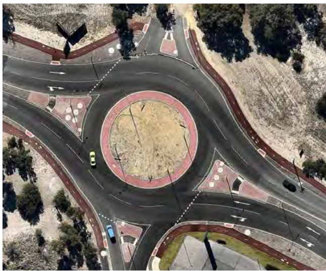
Figure 4.9 Major roundabout example – sufficiently sized refuges allow path users to safely stagger their crossings on the approaches to roundabouts.
