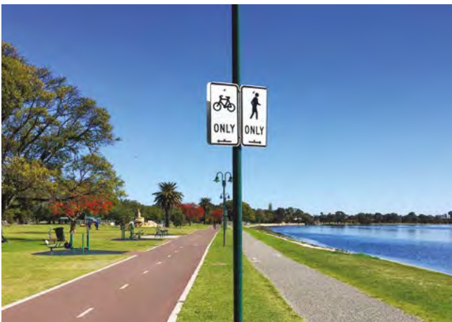
Figure 9.2 R8-3 sign used to formally designate the pedestrian-only and bicycle-only components of a separated path.
