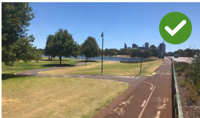
Figure 3.15 Example of clear sightlines at path to path intersection and across curve.
