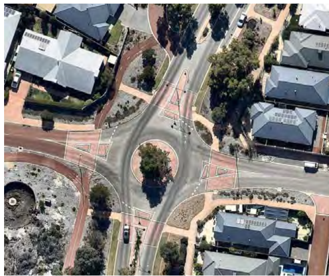
Figure 4.10 Minor roundabout example – sufficiently sized refuges allow path users to safely stagger their crossings on the approaches to roundabouts.
