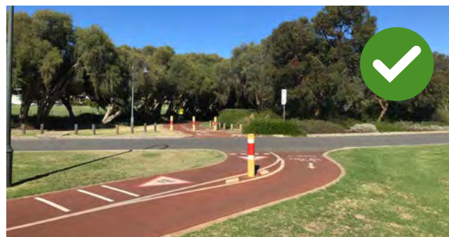
Figure 3.18 Examples of path intersecting at 90 degrees.
