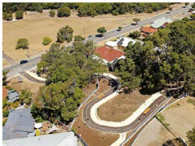
Figure 3.7 Zigzags positioned in appropriate locations could be used to overcome steep gradients (image courtesy of the Wanneroo Times).
