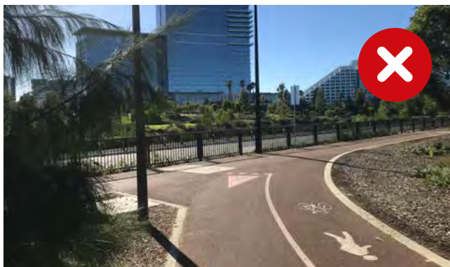
Figure 3.16 Example of poor sightlines at path to path intersection.
