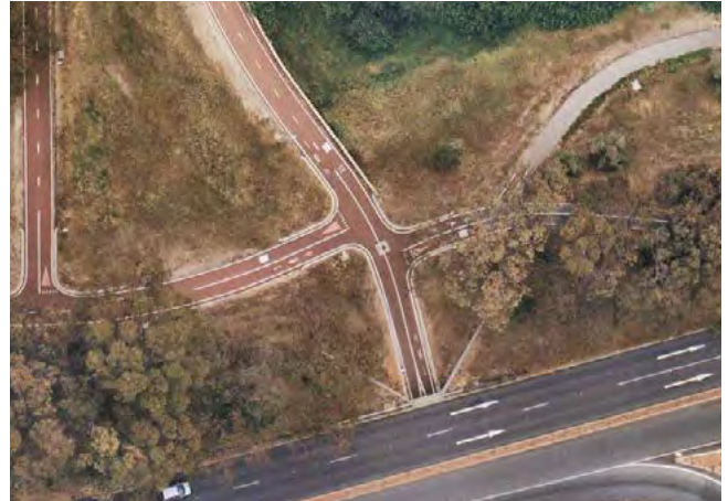
Figure 4.1 Preferred staggered configuration when two paths of equal importance meet.
