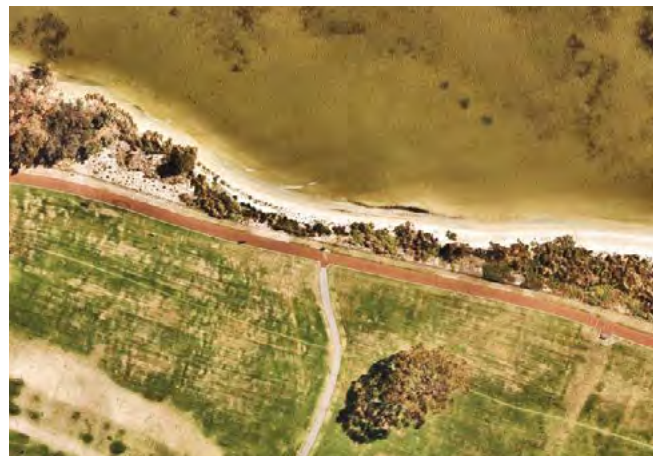
Figure 4.2 Preferred intersection configuration where a high-order path meets a lower-order path.
