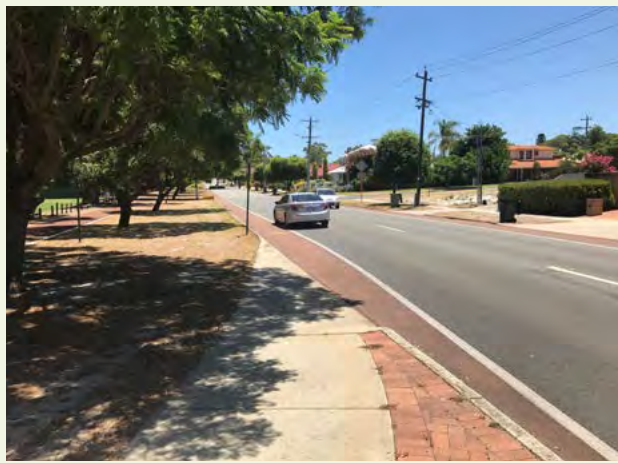
Figure 10.6 Transition ramps from Shared paths to on-road cycle facilities.
