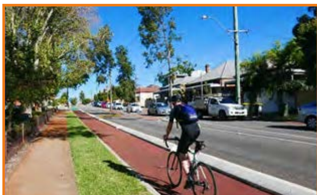
Bike lane protected by concrete kerb
