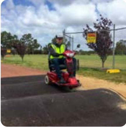
**The impact of speed bumps** was assessed in an offline section of Perth's shared path network to ensure their suitability for the use of wheelchairs and mobility scooters as well as vision impaired pedestrians. This activity preceded the launch of a trial of speed bumps in high-traffic areas.
