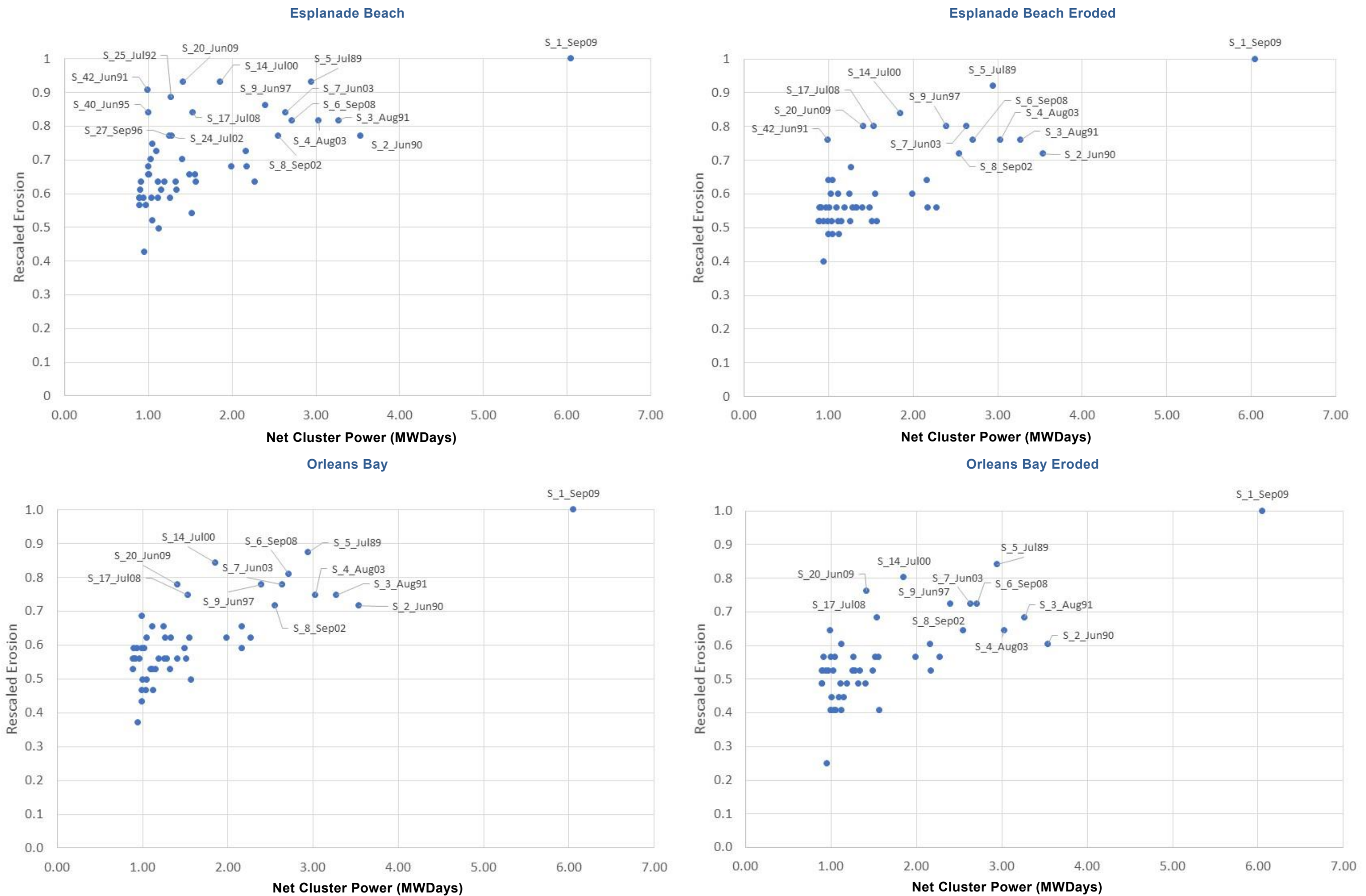
Figure 5.29 Cross Plots of Modelled Profile Erosion versus the Storm Cluster Net Wave Power – Great Southern (Esperance)
